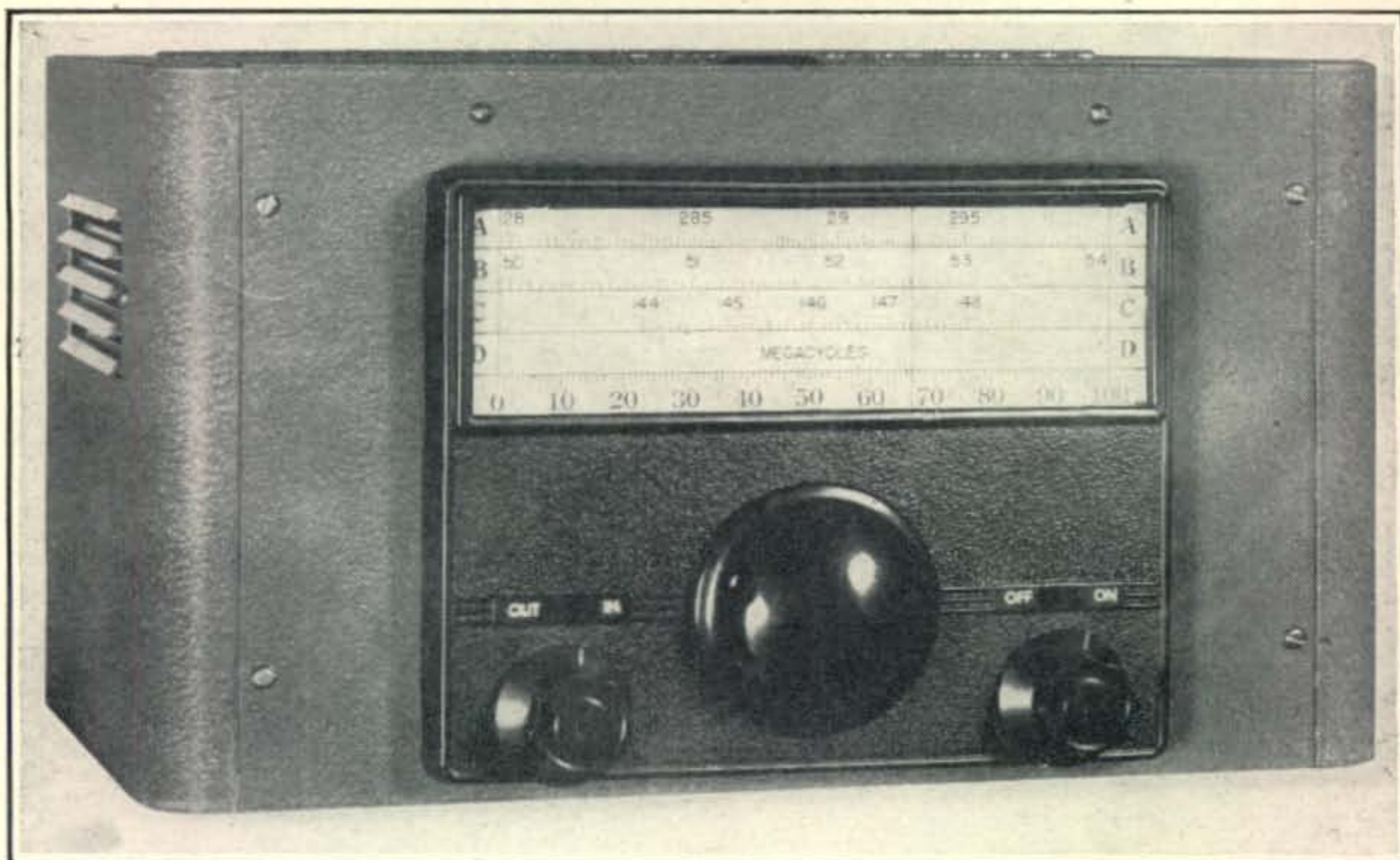
Front view of the three-band converter, shown in its cabinet. The left-hand switch permits the converter to be easily taken out of the circuit while the other control is the on-off switch.
