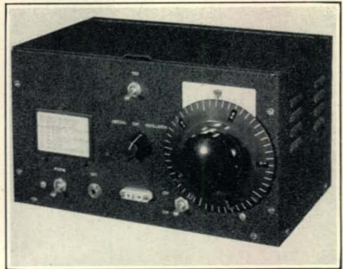
The control unit. The operator selects the desired frequency on the v.f.o. or crystal and presses the key or push-to-talk switch. A switch for spotting the v.f.o., crystal or v-f-o selector, and phone-c.w. switch are the other major controls.
