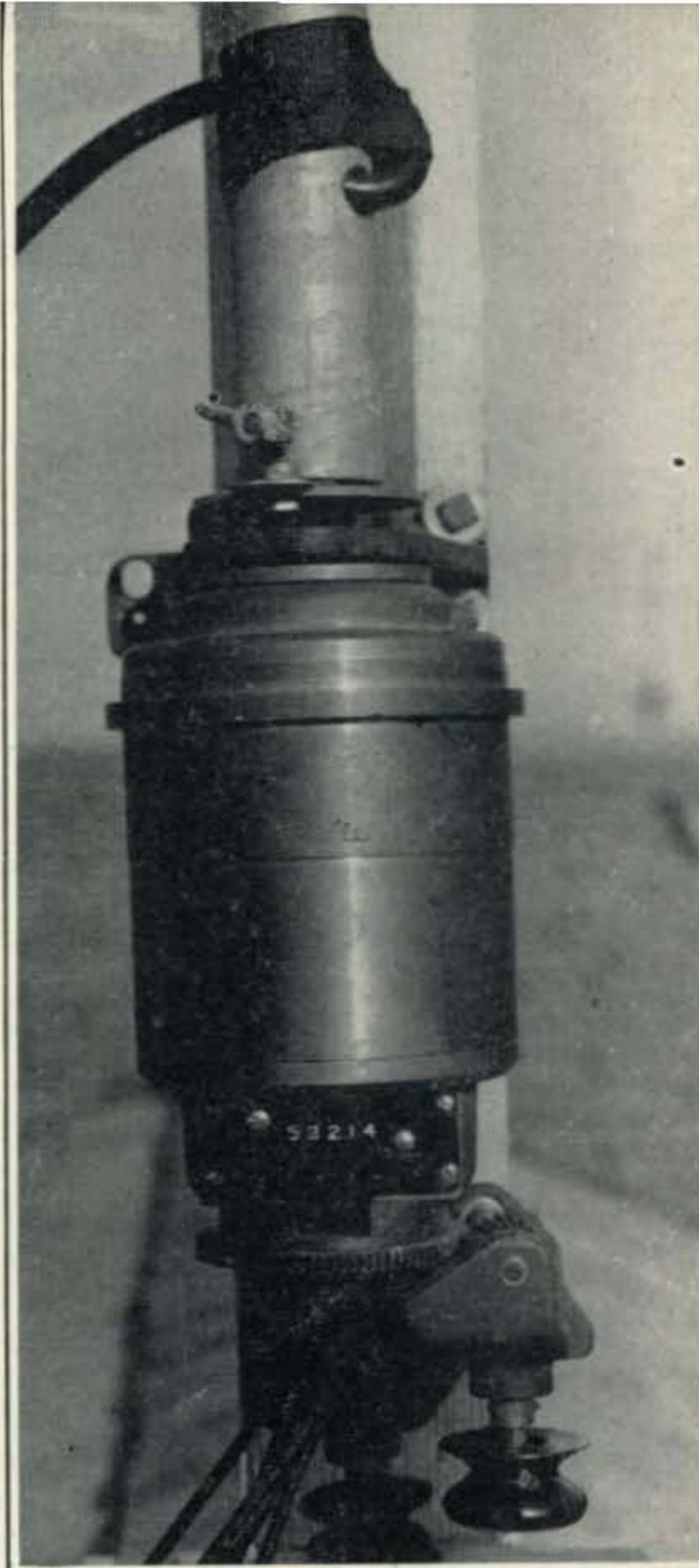
Fig. 3. Closeup of the receiver Selsyn motor used to rotate the entire beam. The motor is mounted vertically and the top bearing serves to support the array. The coax cable is fed through the supporting steel tubing and sufficient slack is left at the bottom to allow two complete rotations. The numbers indicate the five parallel hook-up wires.
