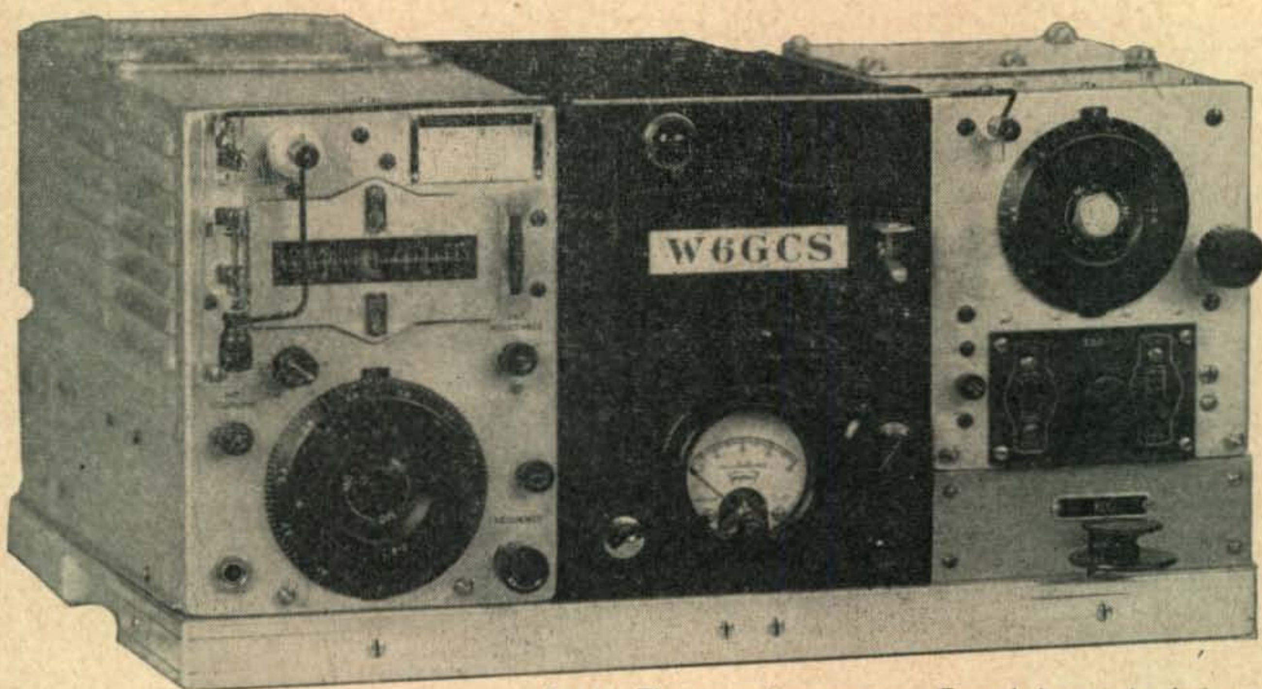
Fig. 1. The complete station. From left to right the units are: transmitter, a-c power supply, and receiver. The hand key is mounted underneath the receiver.
