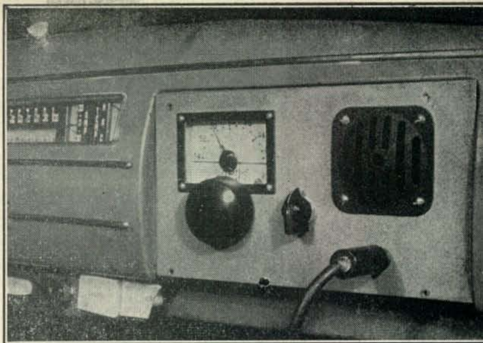
The complete mobile station in the glove compartment of the author's 41 Willys.
