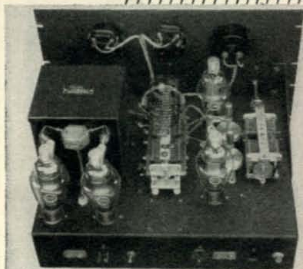
WIPEK's complete 350-w, 3.5-to-28-mc, 'phone/c-w transmitter uses 4 Hytron 5514's — class B and C — and only 7 cubic feet of space. QST for Sept., 1947, pp. 37-46.
