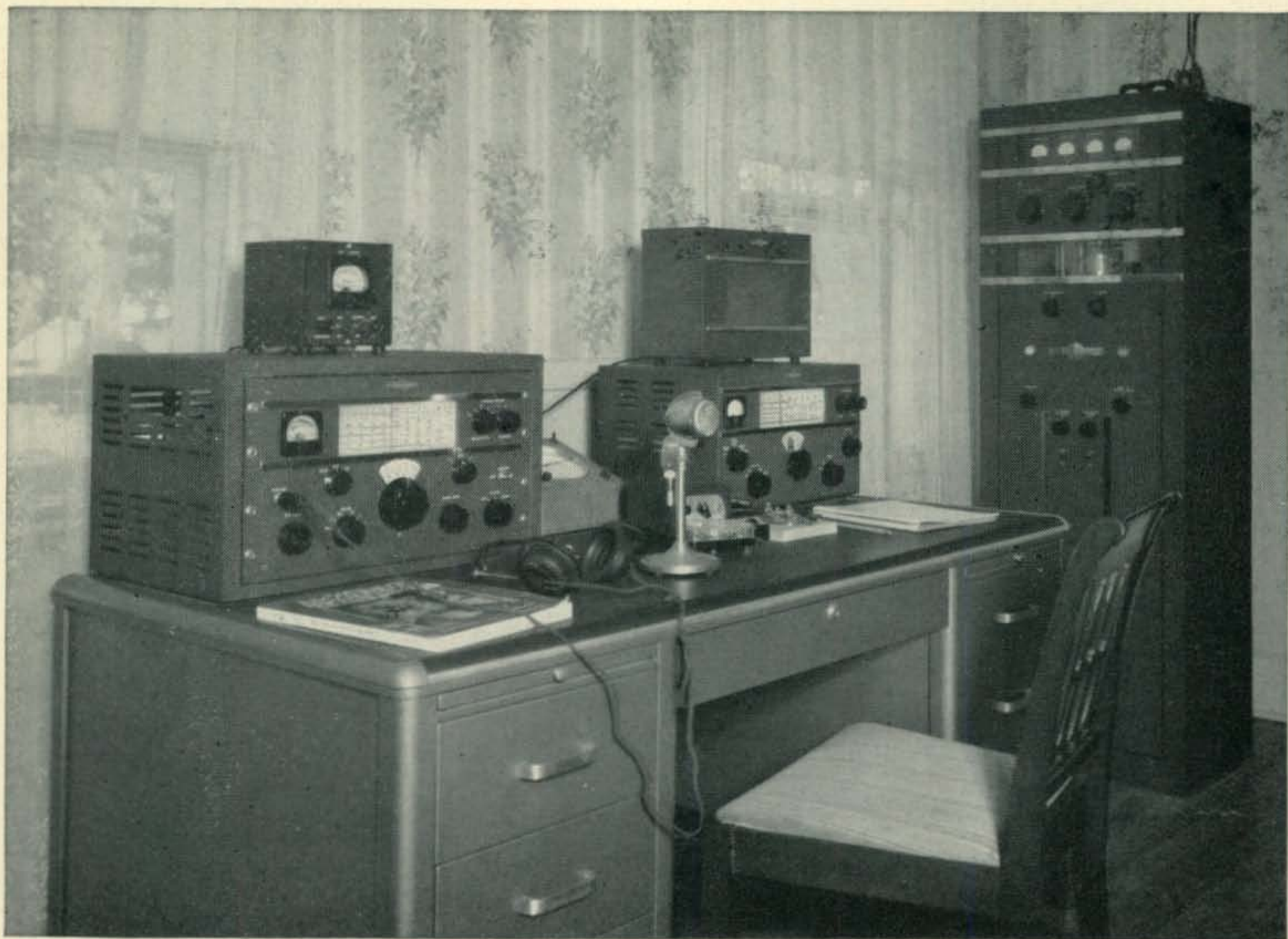
Left to right: Collins 75A-1 receiver, 310A-3 exciter with speaker above, 30K-1 transmitter
