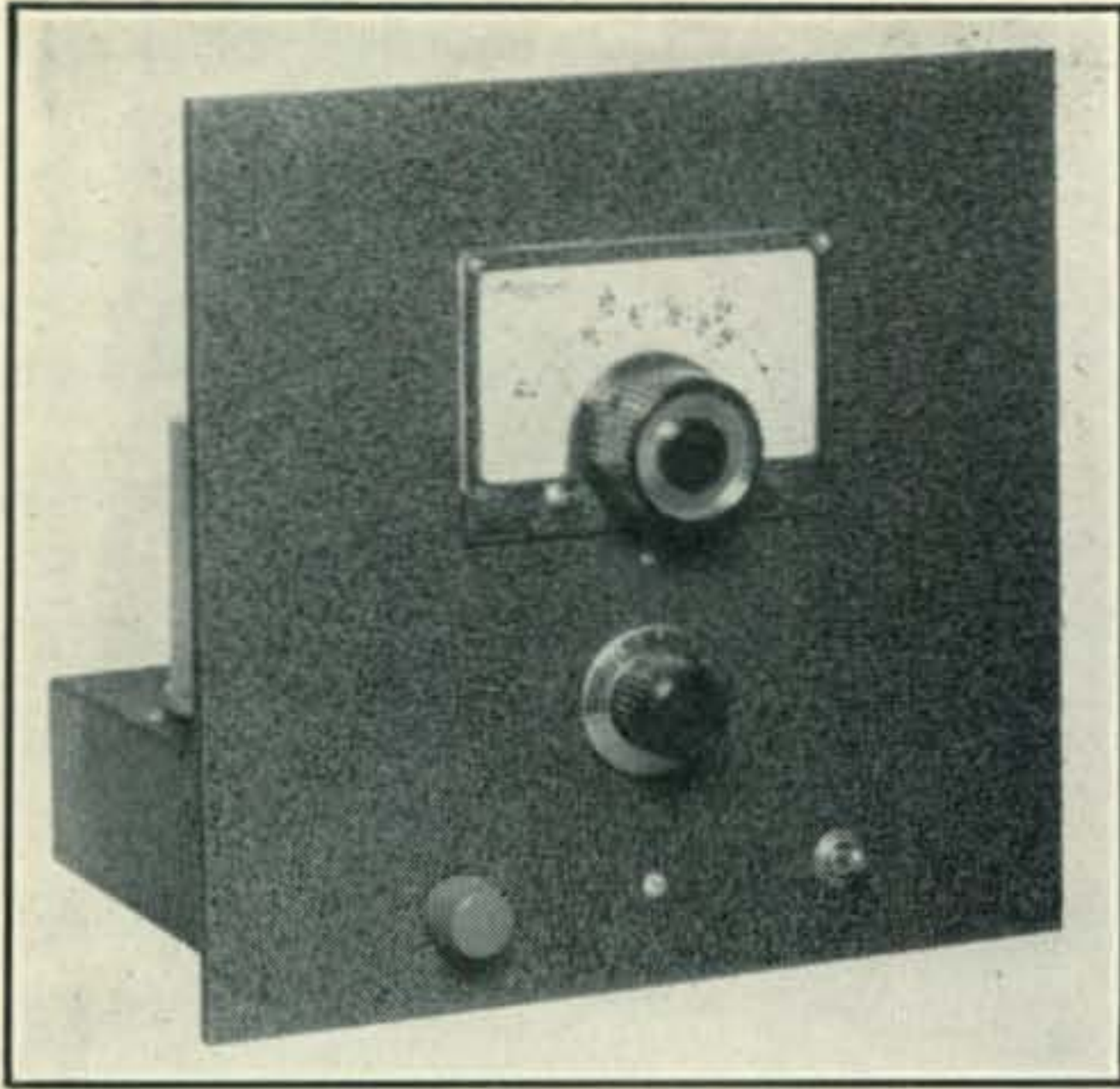
Photograph A. Front view of the beginners' 6, 10 and 11-meter converter. Essentially a single-dial converter, the middle knob is used only to peak the incoming signal.
