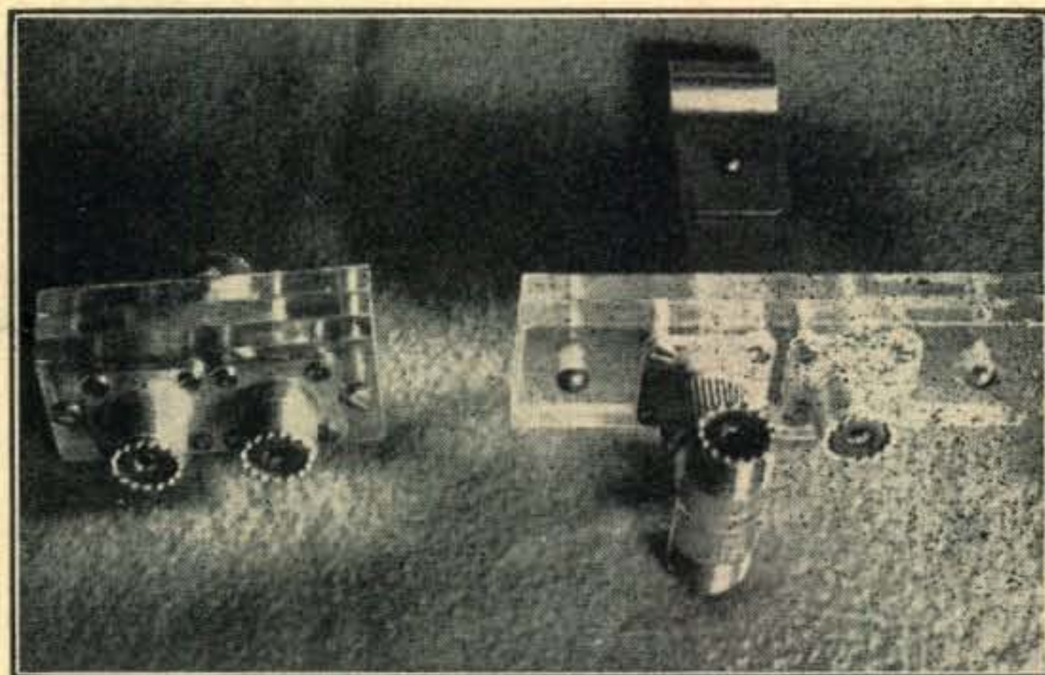
Fittings designed to facilitate connection of coax lines to antenna. The one to the right, designed for a T-match, is illustrated in Fig. 2A; to the left is the coupling shown in Fig. 2B.
