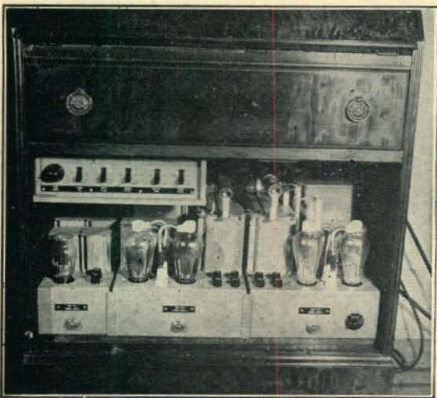
Power supplies with front ventilation louvre removed. Individual controls and lamps are provided for the 600-volt, 1500-volt, and 2000-volt units. A full description of the switching sequence is contained in the text.
