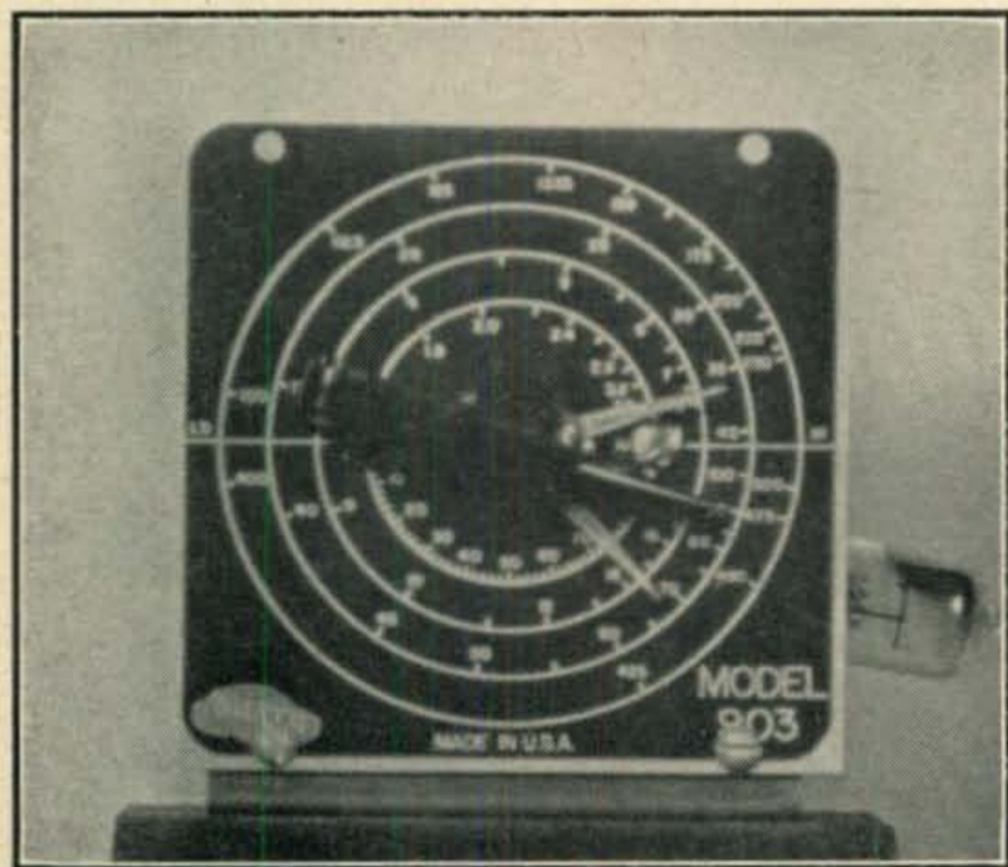
Fig. 5. Two supplementary pointers are added to recalibrate the instrument — one for each set of scales. This setting is for 14.5 or 69 mc.
