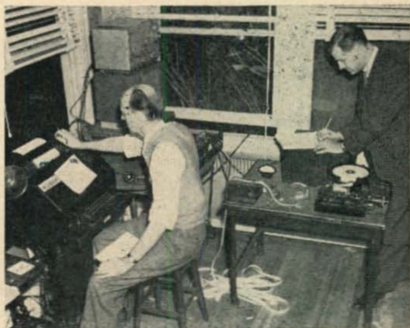
Bill Knott, W2QGH, (left) and Gay Milius, W2NJJ, were kept pretty busy on the teleprinter circuit between the Westchester County message center and WNYC. All of the Westchester election returns went over this 144-mc link.
