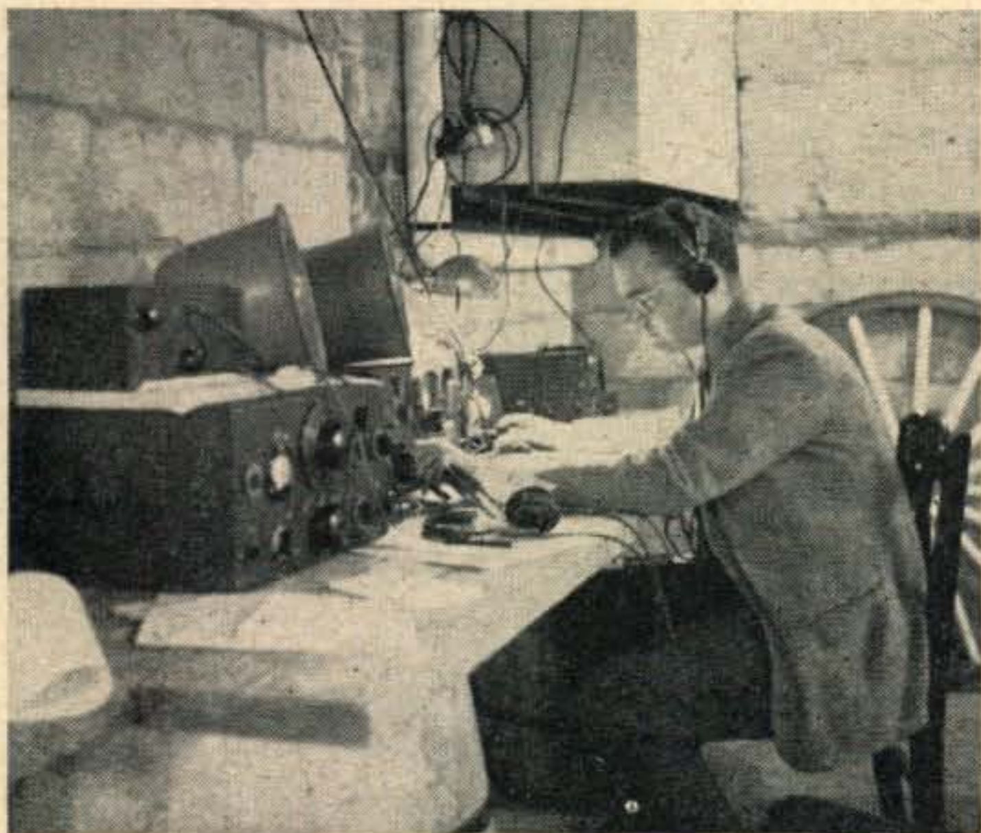
Fred Skinner, W2EQD, operating W2EQD/2 on 3720 kc at the message center. From this point the results were sent down to the finish line on a teleprinter circuit operating on 144 mc.
