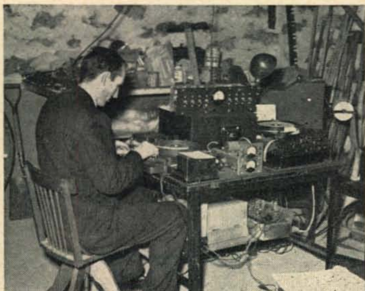
W2BFD spent many busy hours operating his teleprinter installation at the message center. Almost everything was put on tape before transmission in order to ensure "perfect copy" at the receiving point.
