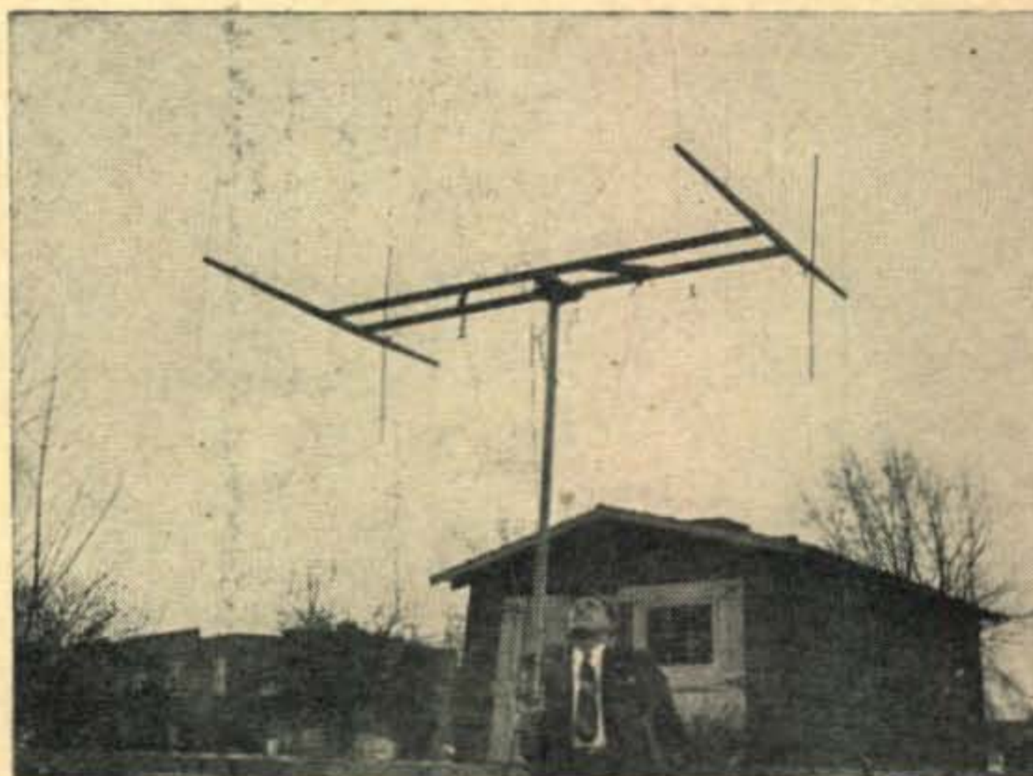
Look, Maw, only one hand! There aren't many 144-mc arrays with a measured gain of around 14 db which can be handled this way.
