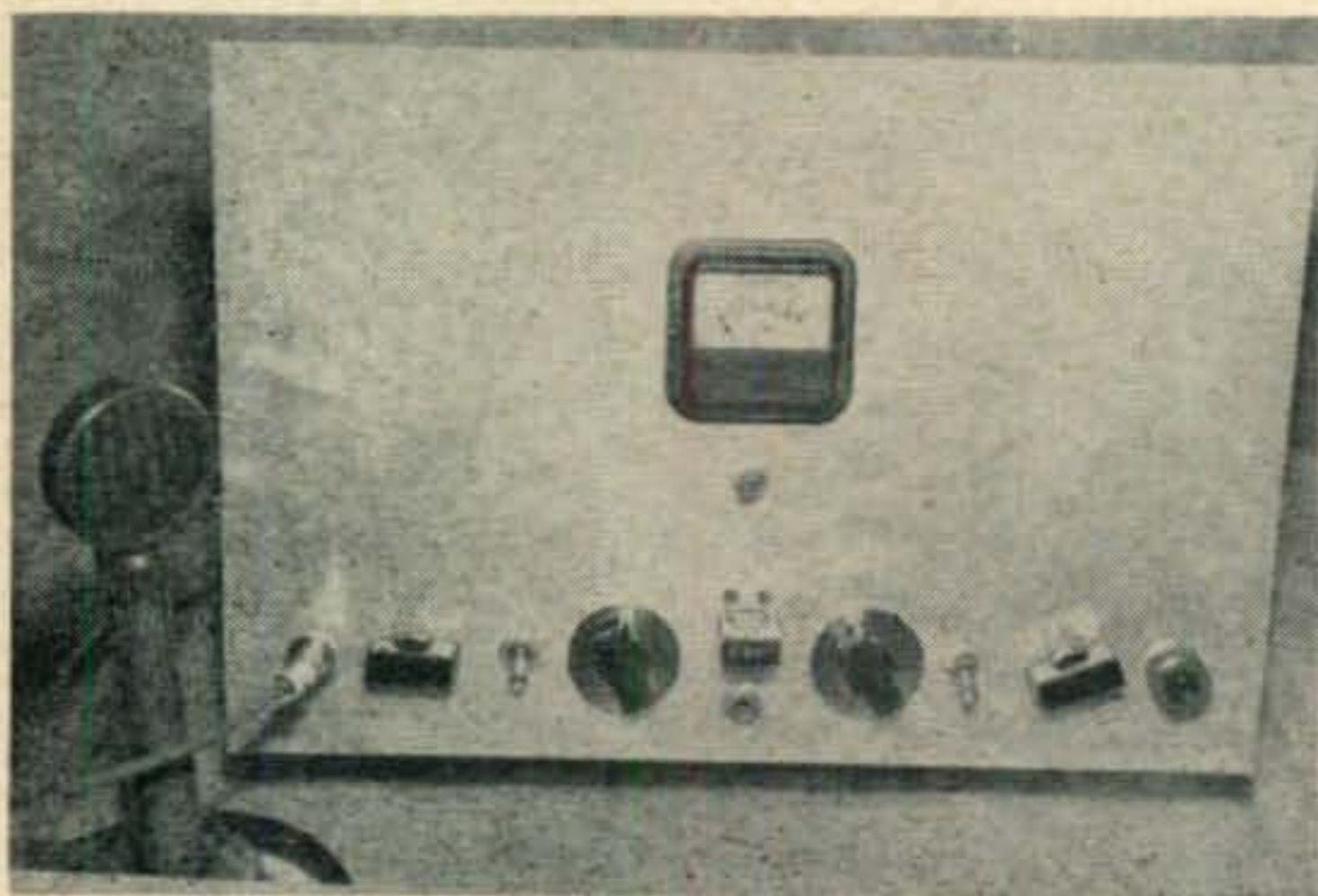
Front panel of the transmitter. The meter switch is directly under the meter. Across the bottom of the panel, from left to right, are: microphone connector, excitation control and a.c. switch, keying selector switch, oscillator tuning, B-switch, audio gain control, and pilot lamp.
