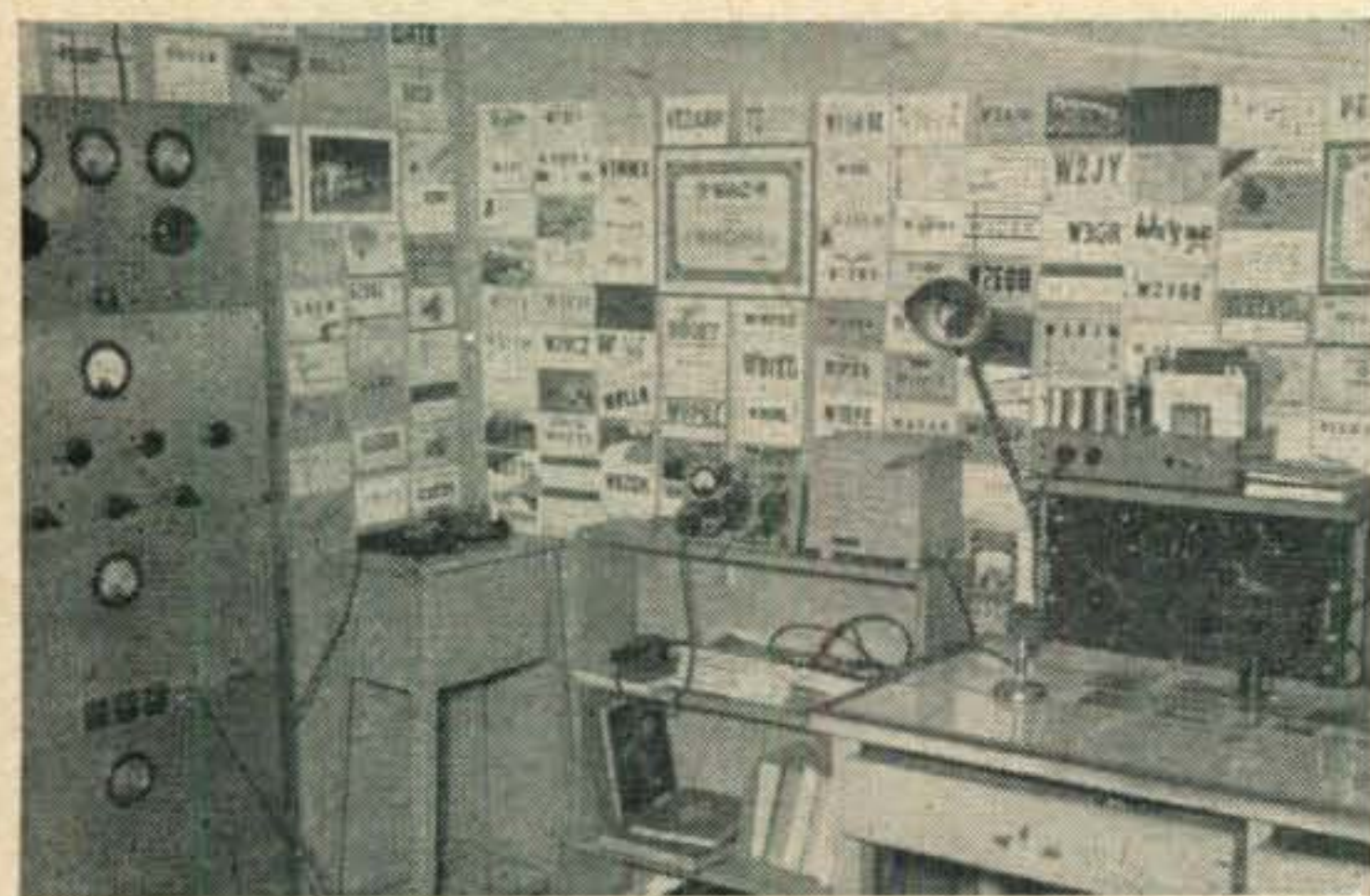
The operating position at IIRC/Trieste. An 828 occupies the final seat in the transmitter, while a BC-312M, behind a converter, does the receiving.
