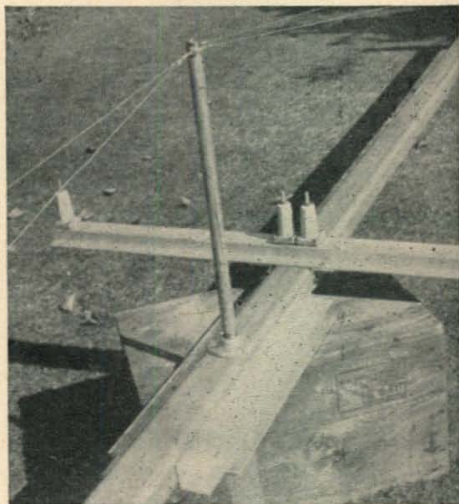
The beam mounting plate attached to the boom, illustrating the top guys and the method of mounting the support for the driven element.
