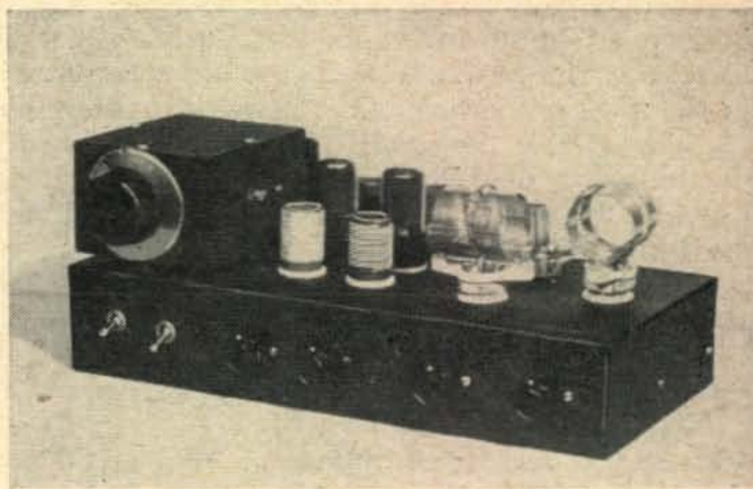
The National dial on the penthouse at the left controls the operating frequency. The multipliers and their attendant coils are visible just to the right of the VFO box, and the final tank and antenna coils are at the right.
