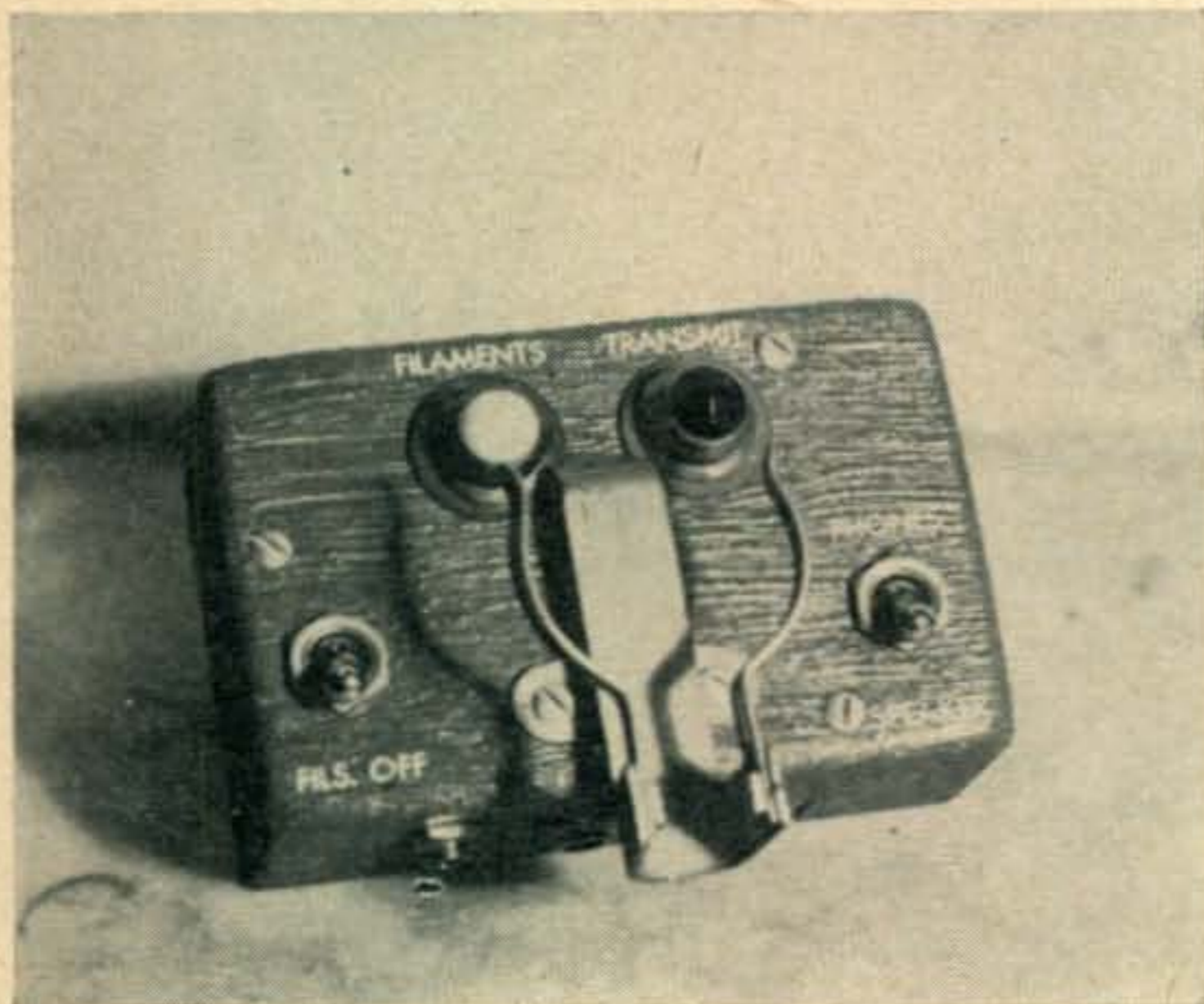
The control panel. The phone and mike jacks can be seen on the underside.
