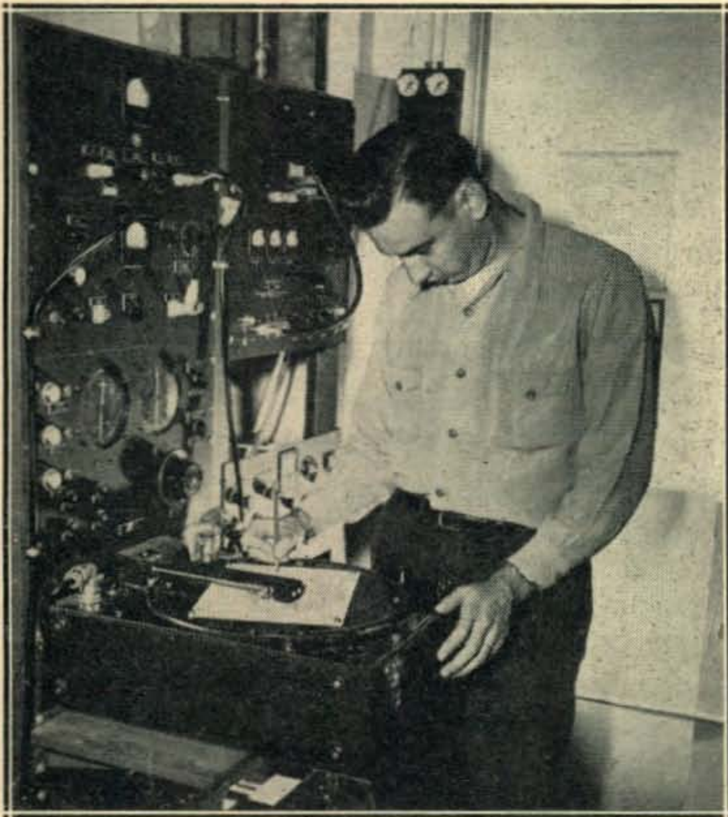
As the airplane model is rotated in the setup shown on our front cover, the antenna pattern is automatically traced out by the polar pattern recorder.
