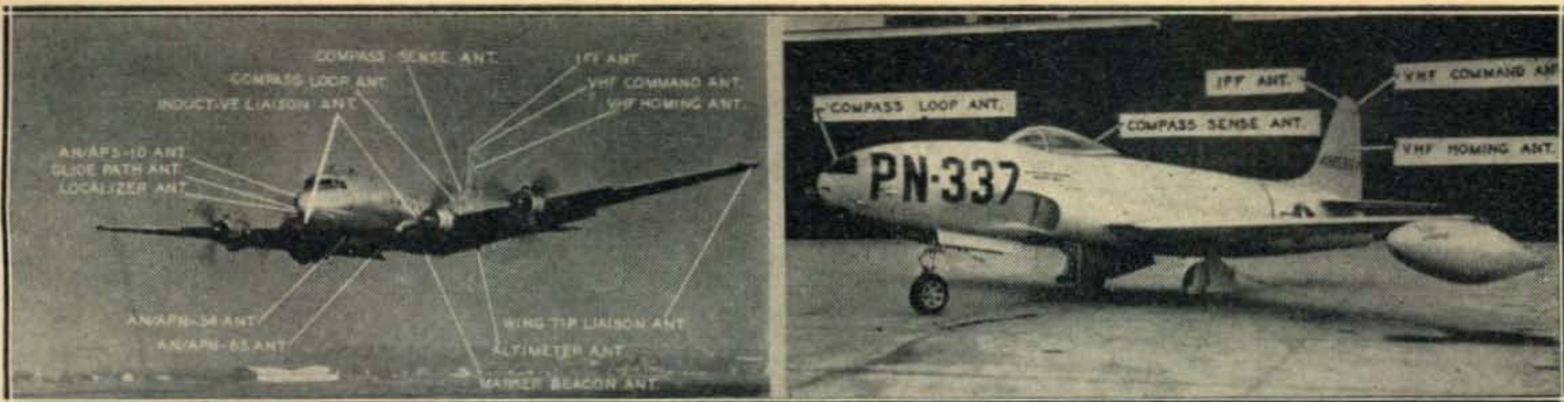
Left: There are more than a dozen antennas buried under the skin of a C-54. The elimination of "drag" in this case saves several hundred horsepower. Right: The F-80 fighter has five buried radiators, including three in the tail (vertical stabilizer).
