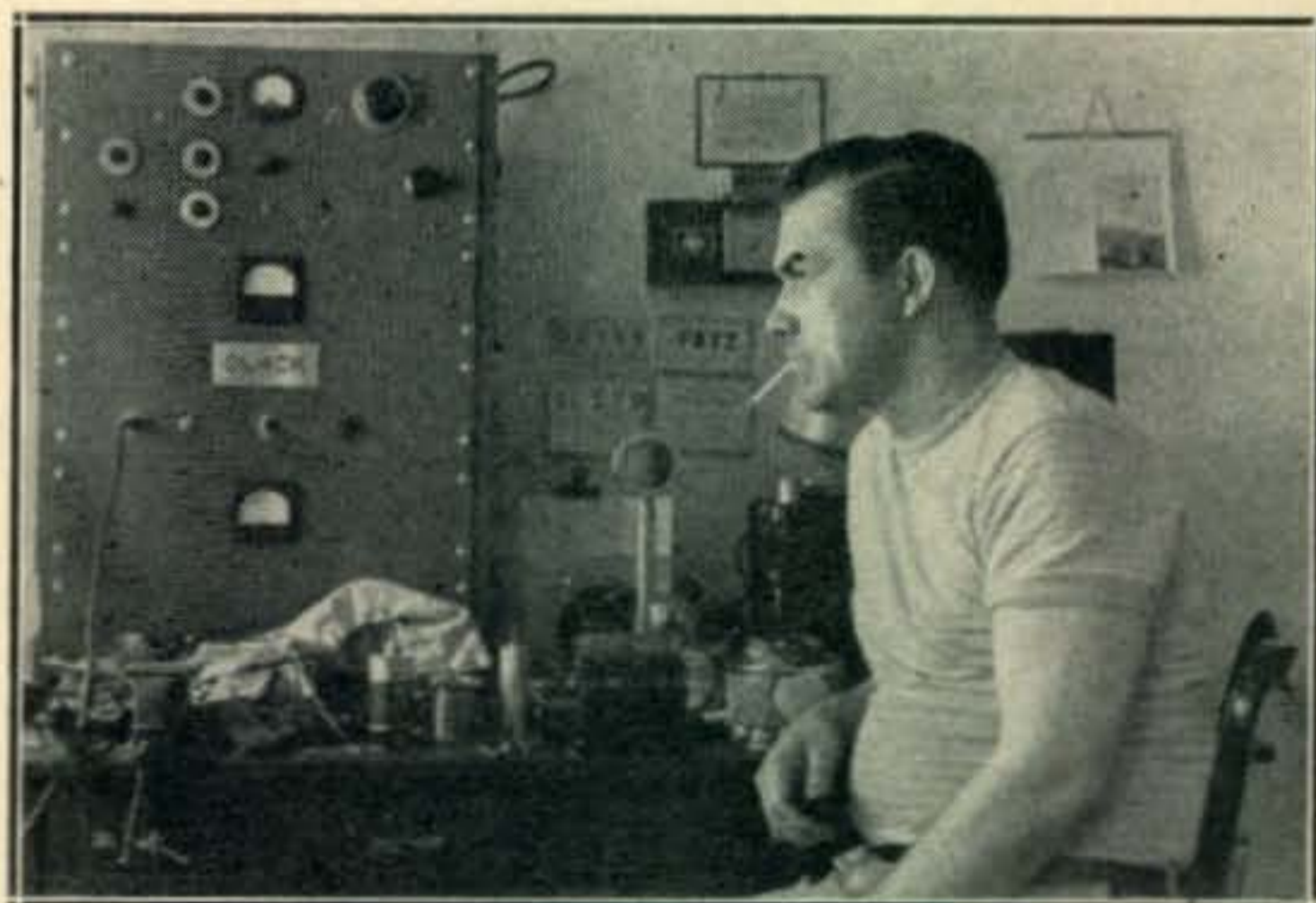
The operating position at DL4CK, Wiesbaden, Germany. Note the weather-warning instruments on the wall! All these DX QSLs are from two-meter operation. The present receiving set-up uses a Wallman Cascade converter into a BC-342.
