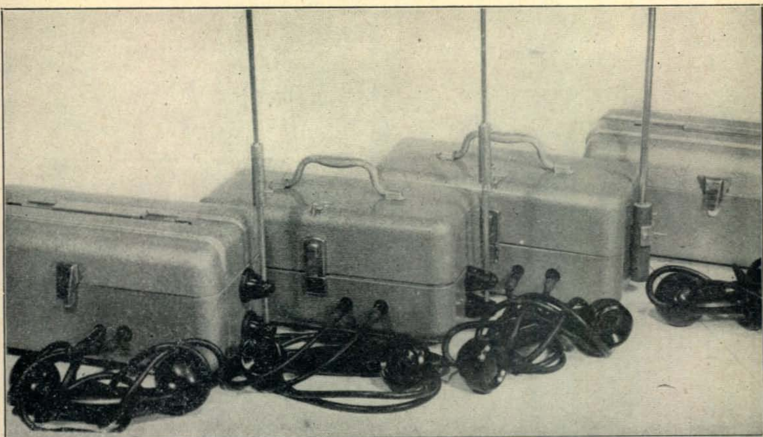
Four of the Norwalk Red Cross 28 mc walkie-talkies. Note that two different styles of fishing tackle boxes are used. Cables for the handset are plugged into the chassis through holes in the side of the box.
