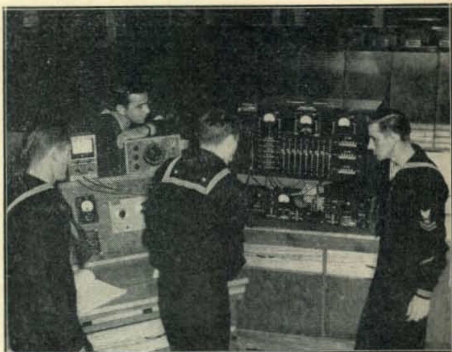
Power in parallel circuits being explained by use of circuit demonstration panel.
