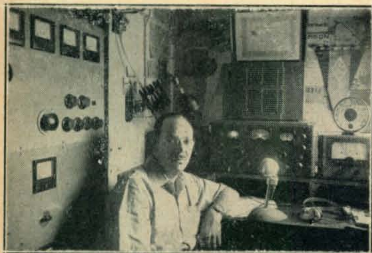
Romulo Fabres (EA3FL) at the home station uses a pair of 813s at 600 watts and a 3-element rotary beam.
