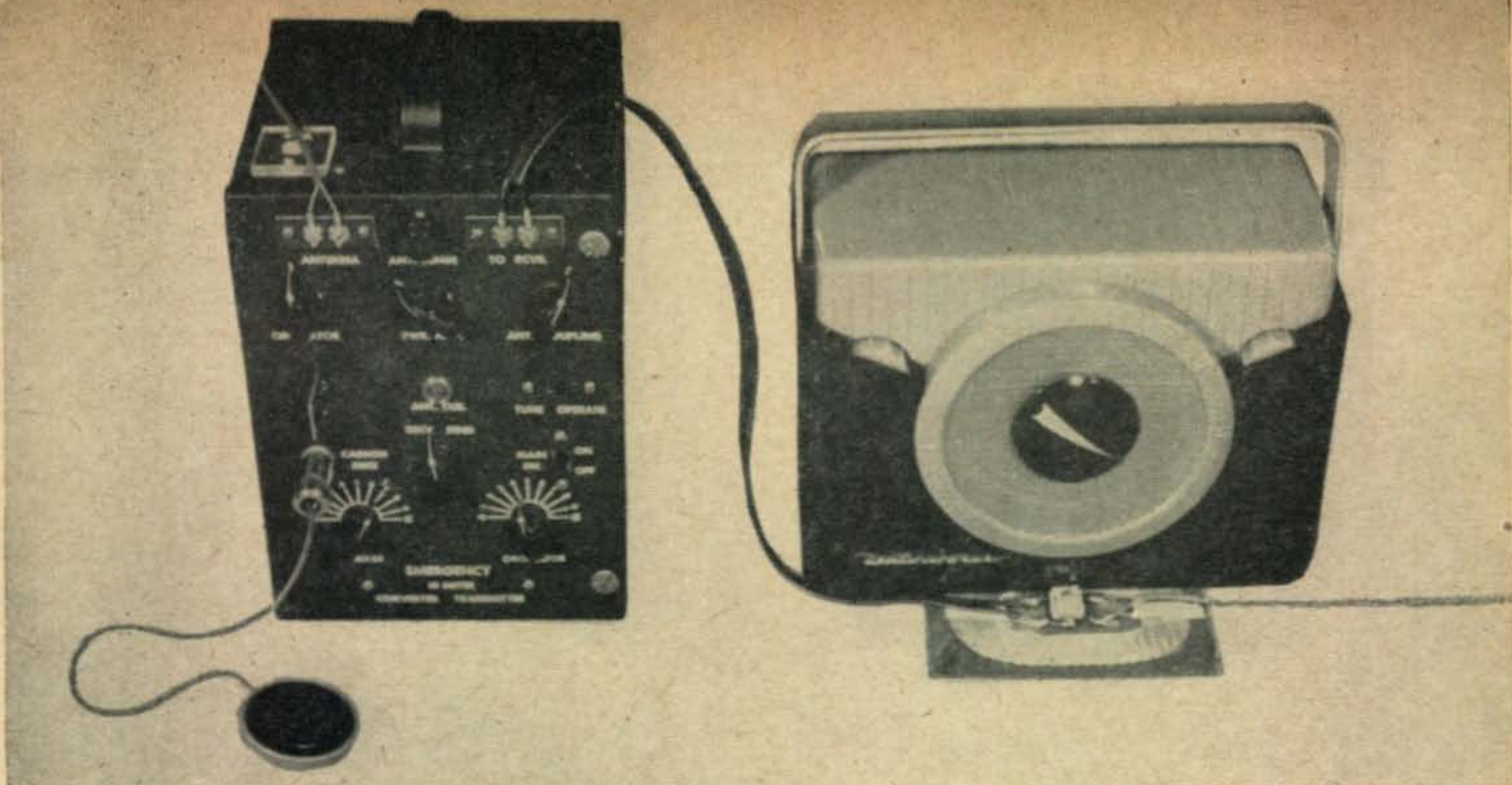
The complete emergency station featuring a self-contained transmitter and a 28-mc converter. The converter is loop coupled to any battery BC receiver. The microphone is an F-1 cartridge with leads soldered directly to the contact rings.
