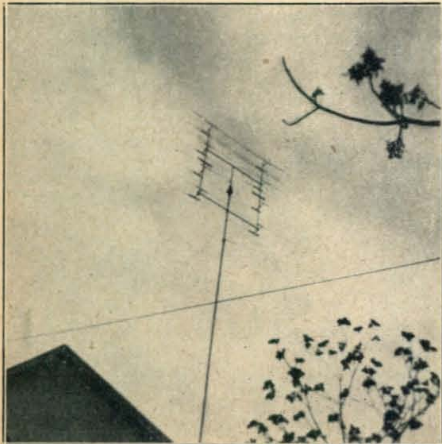
Antenna at WN8HOH 32 elements 53 feet high at 730 feet above sea level.
