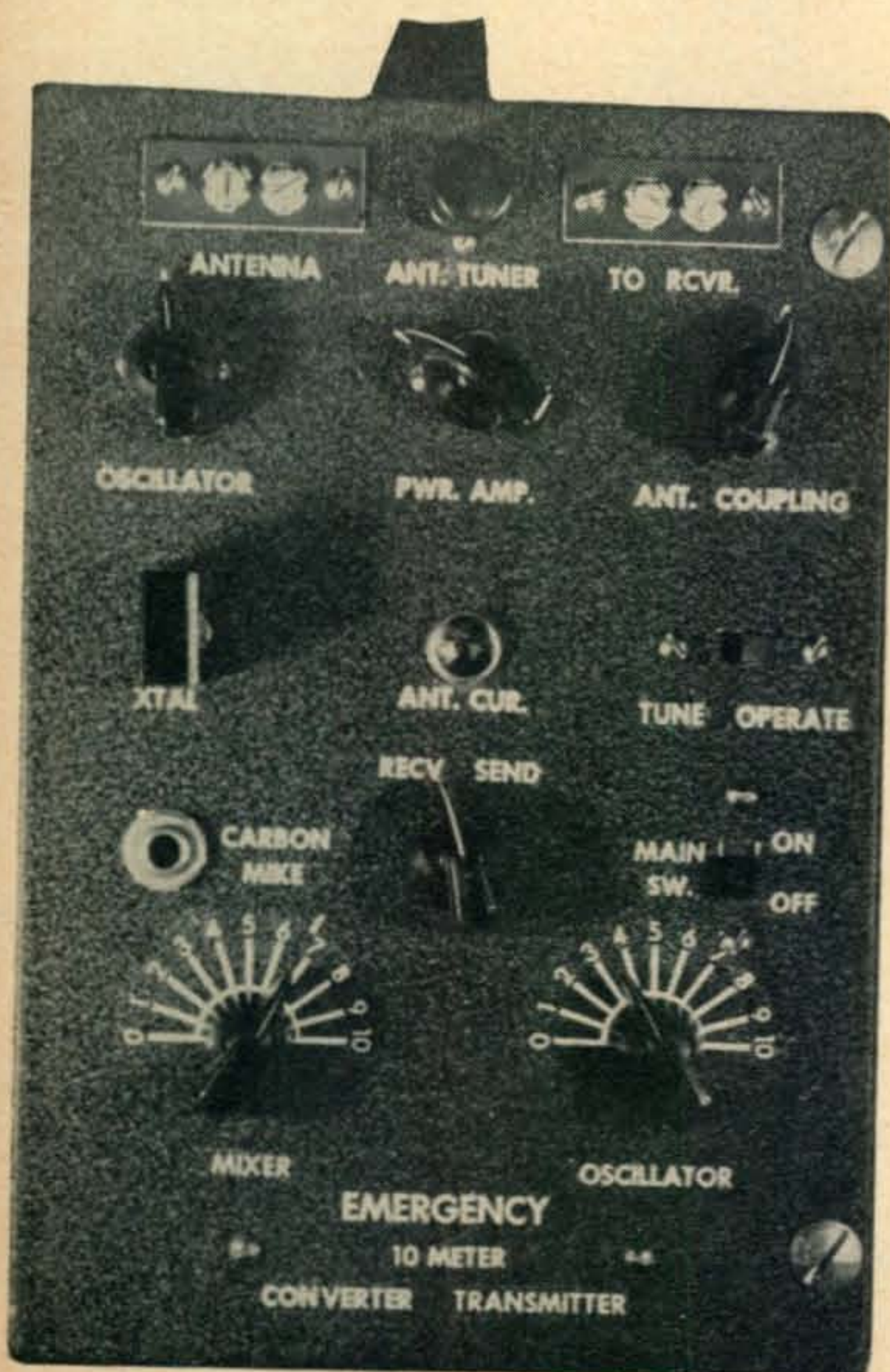
The front panel is completely marked in case the unit is placed in the hands of an inexperienced operator.
