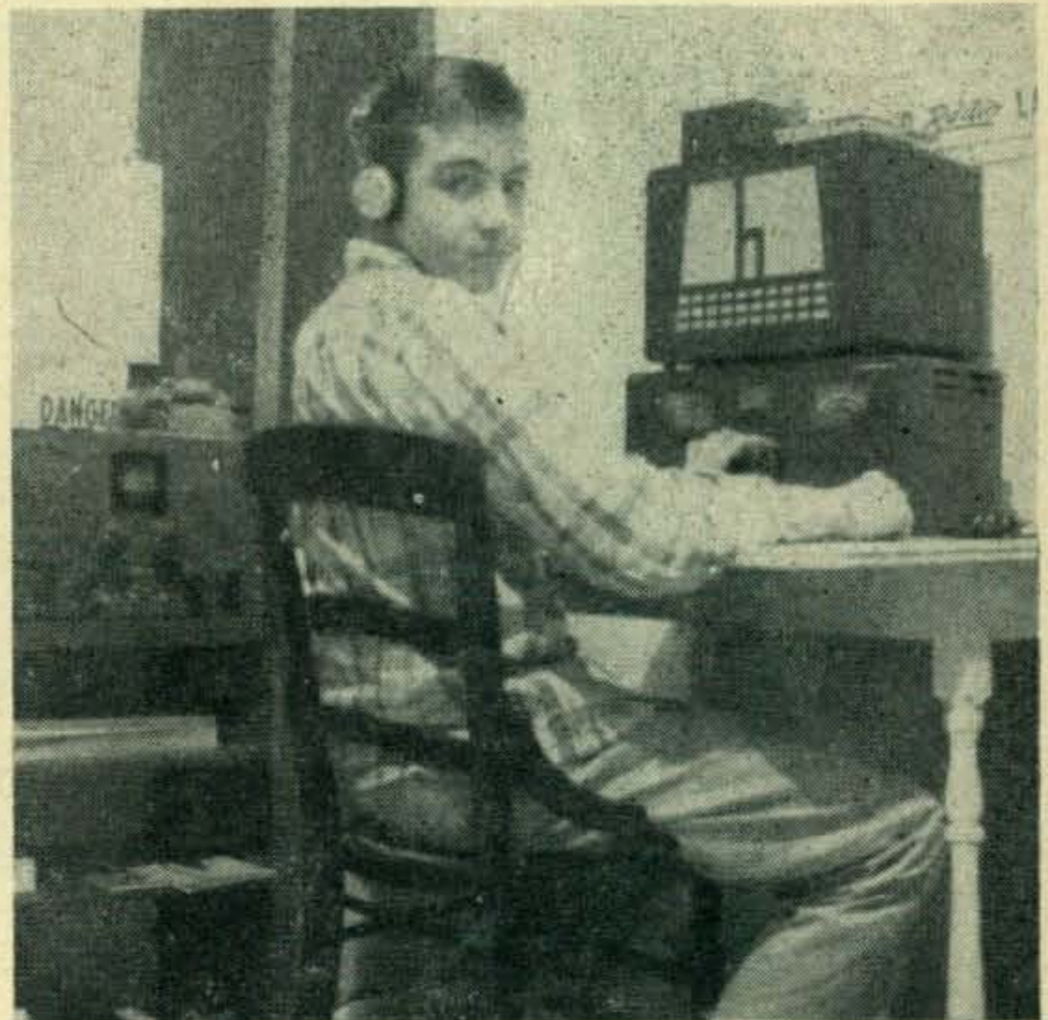
WN5TOM, Louis E. Frenzel, Jr., Galveston, Texas. The transmitter is a 6AG7 with 11 watts input. Receiver is an S-76, with an S-20R for a monitor. Long wire antenna. Louis is thirteen and in eighth grade. He has worked 26 states.
