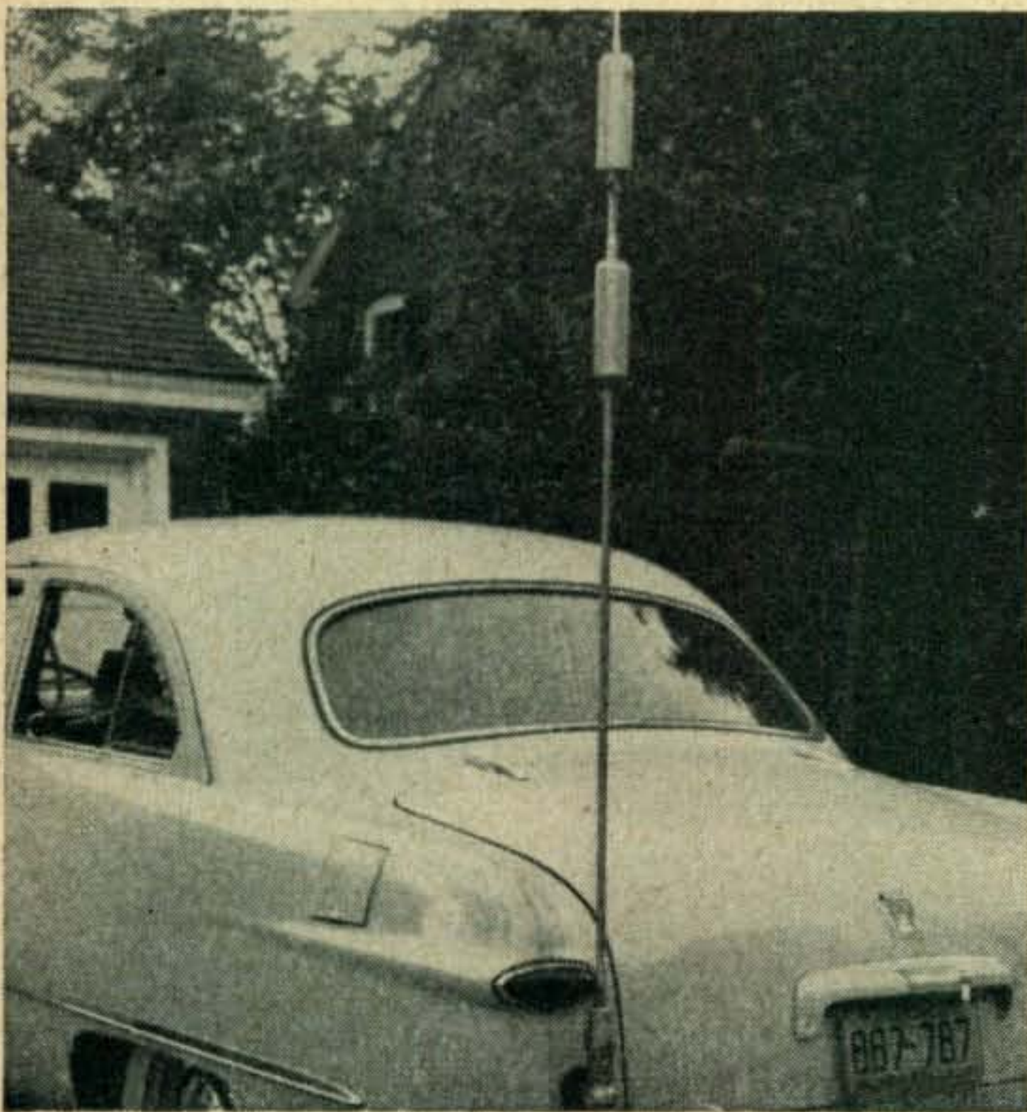
Multi-band operation requires the use of two loading coils—one for 20 meters and one for 75 meters. This is the installation of WØEMM who describes a transmitter elsewhere in this issue.
