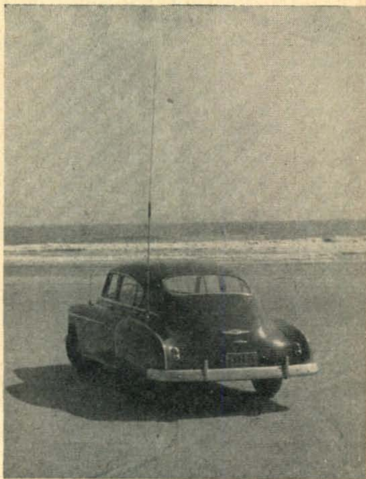
The author's Chevy contains a three band installation using only war surplus materials. The antenna is the usual center loaded 75 meter whip.
