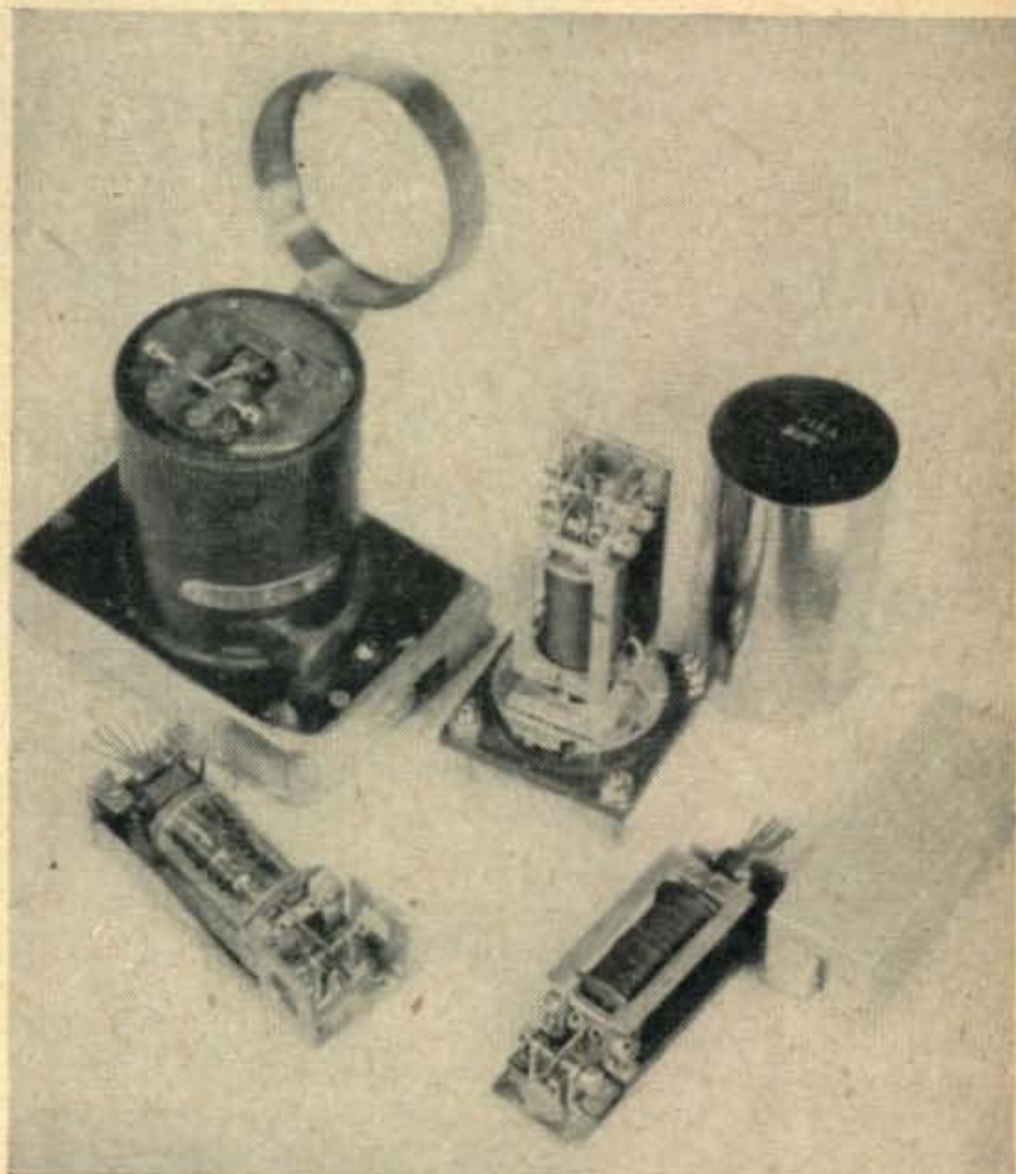
These are a few of the polar relays commonly found in teletype equipment.
