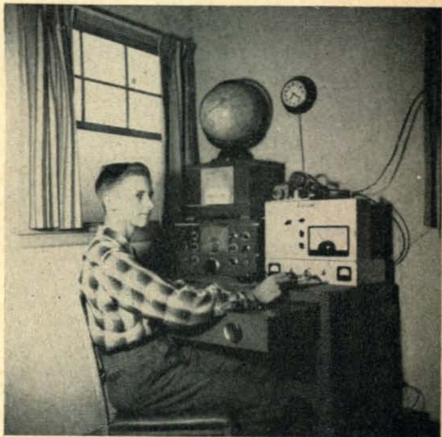
The neat station of Dick Powell, W8IJM, who recently graduated from the Novice ranks. The transmitter ends up in a pair of 807s. The receiver is a National NC-240D. Dick is fifteen years old and in the ninth grade
