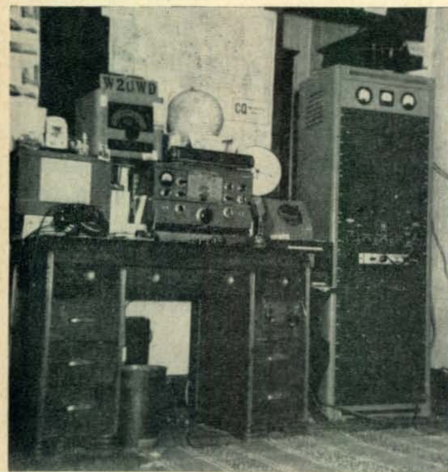
Familiar to all are the husky signals of W2UWD, Bob Turrell, of Binghamton, N. Y., which emanate from the rig pictured above. Bob runs 700 watts on all bands with rotary beams on ten and twenty. Receiver is an NC240D and a DB22A.
