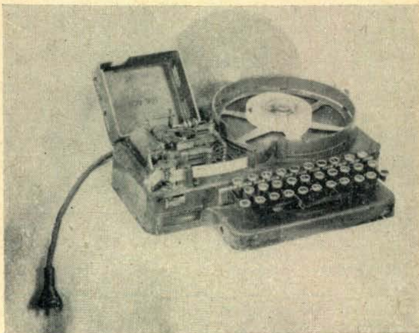
A keyboard perforator for punching teletype tape.
