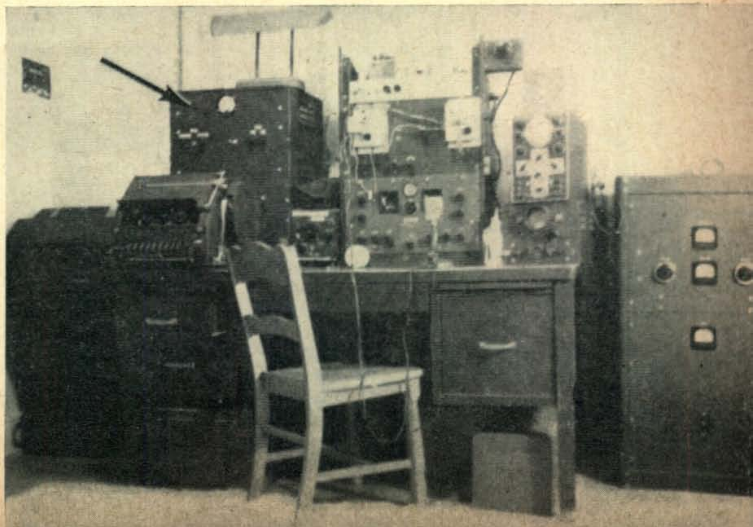
This is the outfit at the Author's Shack. The Receiving Adaptor is in the top of the Cabinet (indicated by the arrow).
