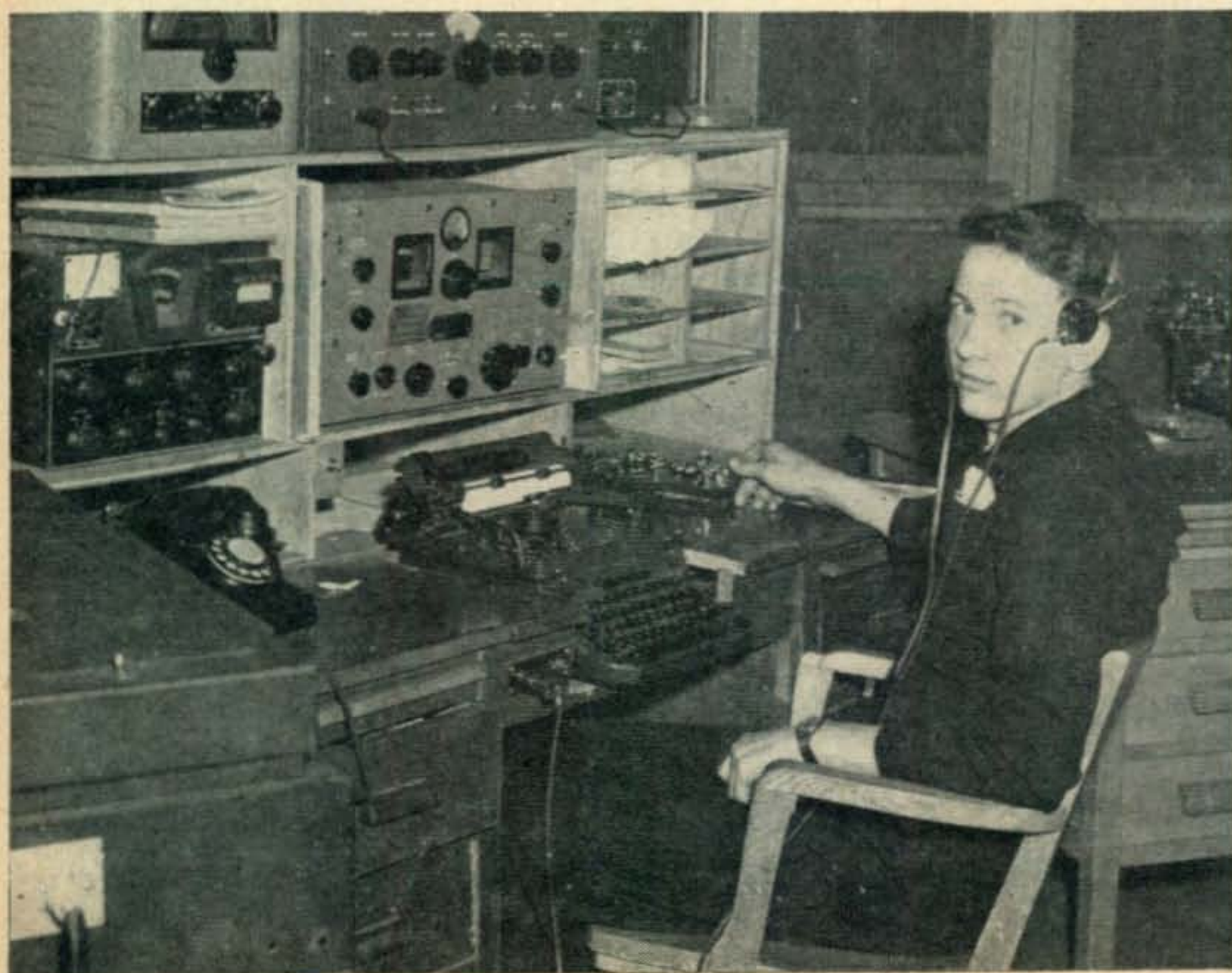
Jim Elgin, CT3, USN, WØCMU, traffic manager, Navy Mike and Key Club, Far East, operating the club station, JA2KW. The station consists of a 32V2 driving a BC61OE on 14 mc. On 28 mc. the 32V2 is used by itself.
