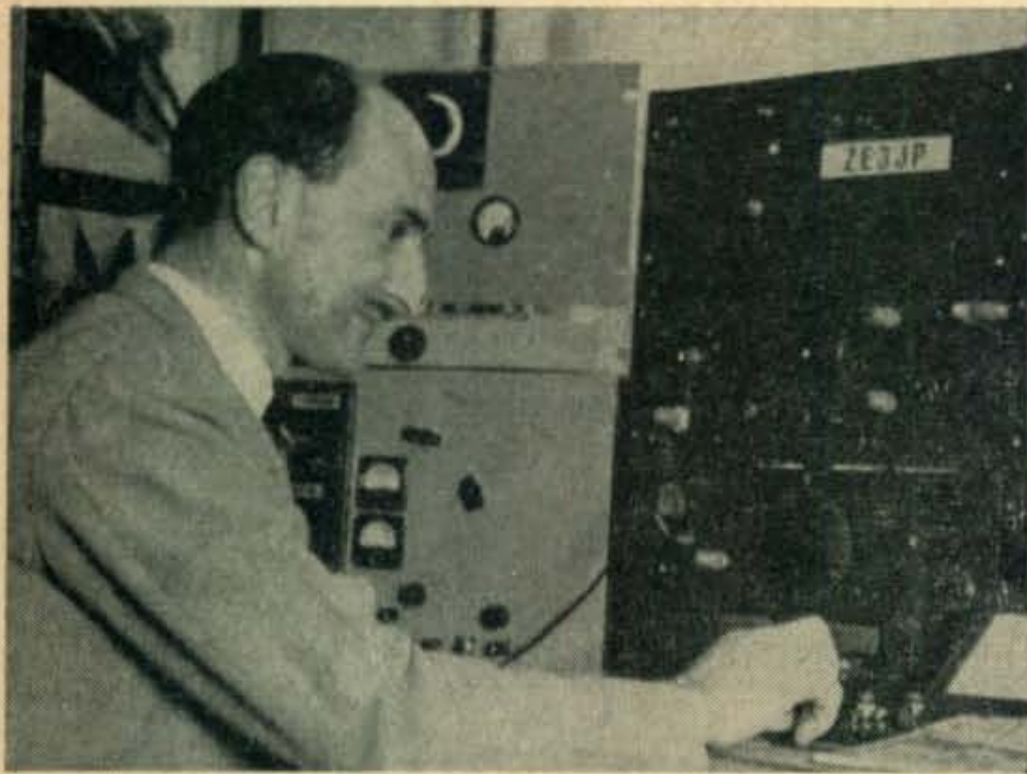
ZE3JP made 103,545 points. Rigs use an 813 and 257B as finals. Receiver is a prewar HRO. Dipoles are used for each band plus a 3-element beam on 10 meters.
