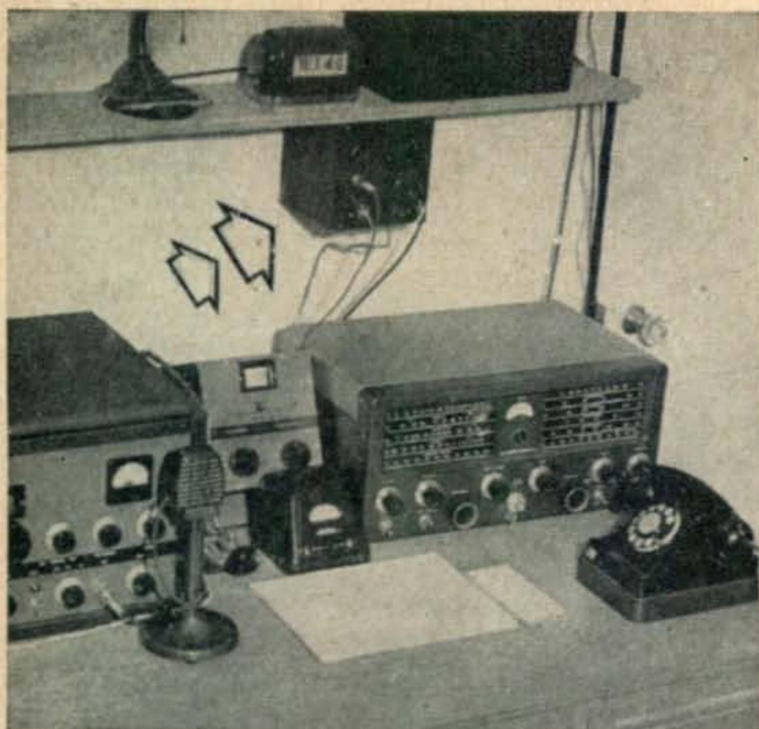
The 'patch' is conveniently mounted just above the operating position and within easy reach of the telephone and transmitter.
