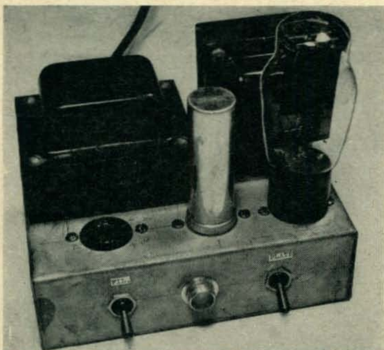
Power Supply used with the Novice phone transmitter. The empty socket is the female connection for the output voltages.
