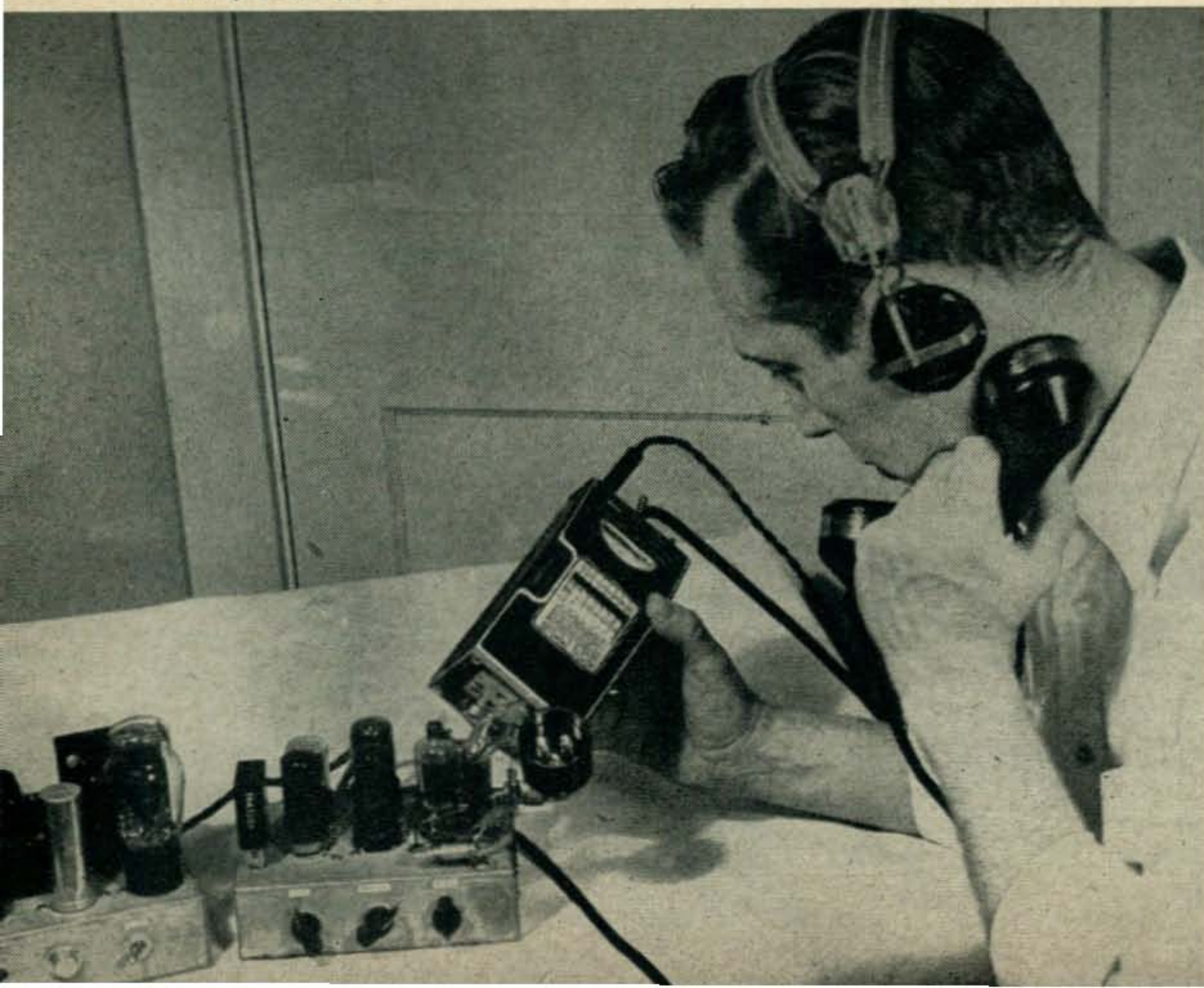
Here W2SPV is using a grid-dipper as a non-oscillating detector to check the modulation quality of his 144-Mc transmitter, described elsewhere in this issue. The dipper coil was placed quite close to the final coil in order to insure that the actual output signal was being monitored. The circular box in the antenna jack of the transmitter is a dummy load.
