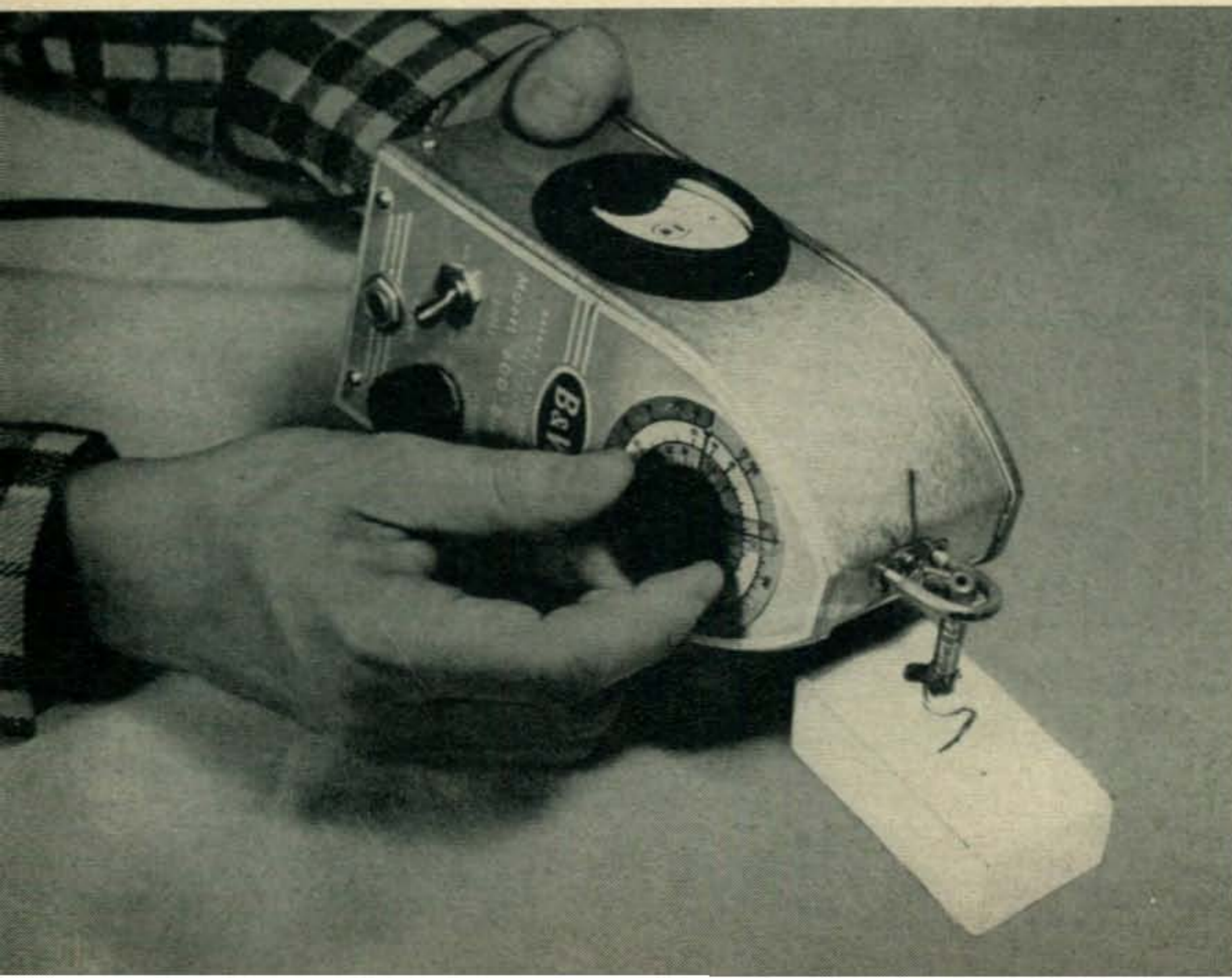
This is the method of determining the natural resonant frequency of a common v.h.f. r-f choke coil. In this case, the choke is acting as a parallel-tuned circuit, in which the capacitance is formed by the stray capacitances between the individual turns of the coil. Note that both ends of the coil are insulated from ground and dressed away from grounded objects. This choke had a pronounced dip at 130 mc.
