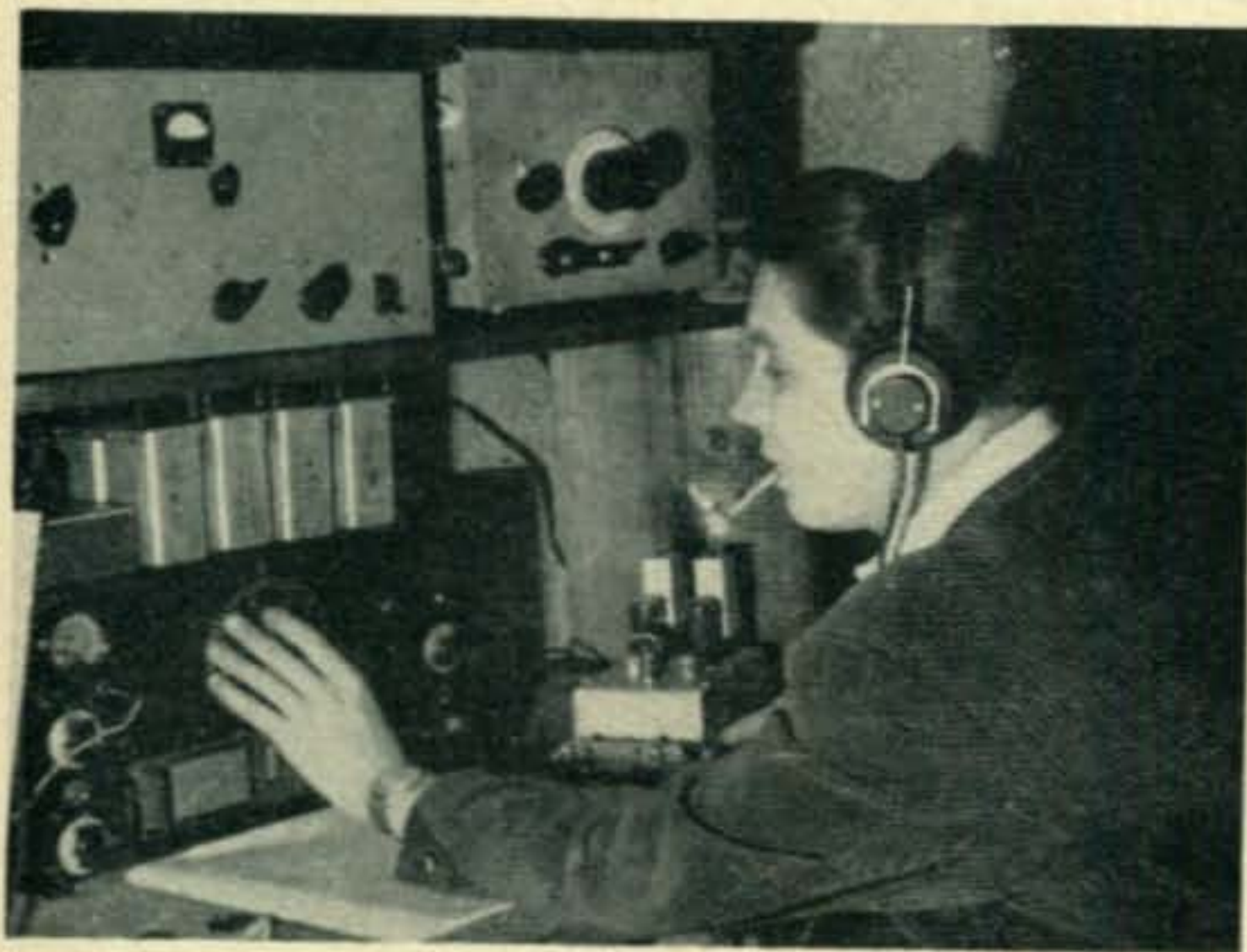
Active on all bands is YUIAD of Belgrade, Yugoslavia. Mirko runs 250 watts to an 813 and has worked 191 countries including 61 on 3.5 Mc. alone. Two ground plane antennas are used on 14 and 21 Mc. and a vertical dipole on 28. Mirko's smooth fist is helped by the W6DPU el-bug which may be seen at lower left.
