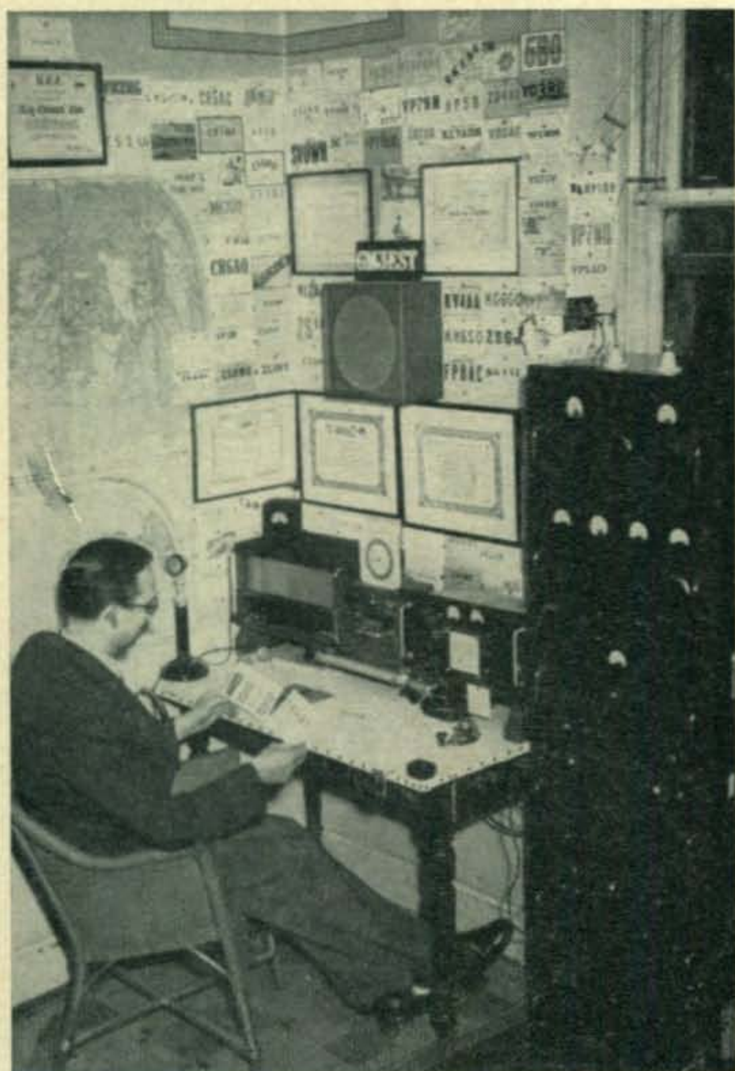
The neat layout of Andrew Sinclair GM3EST, which is single-switch controlled and equipped for full break-in working on CW. The rack on the right ends with an 813.
