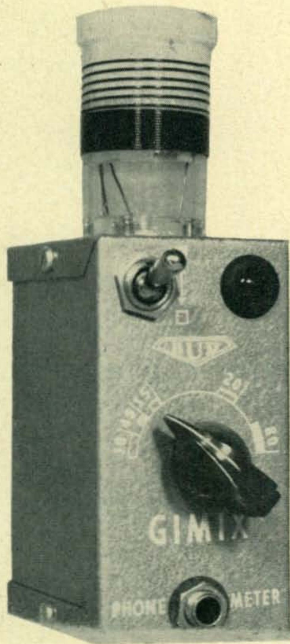
Bud GM-79 Wavemeter reviewed in this month's column. It sells for approximately nine dollars.
