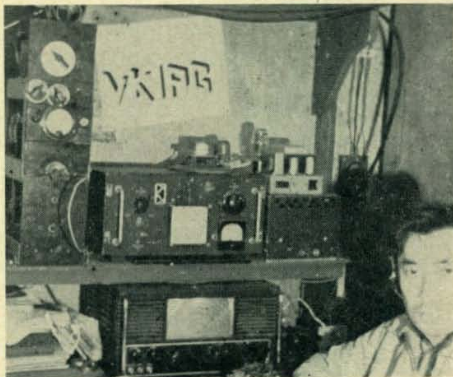
This is VK1FG at Heard Island, Antarctica 1950. The rig was a pair of 807s modulated with 6L6s. The receiver was an Eddystone (British) 680.
