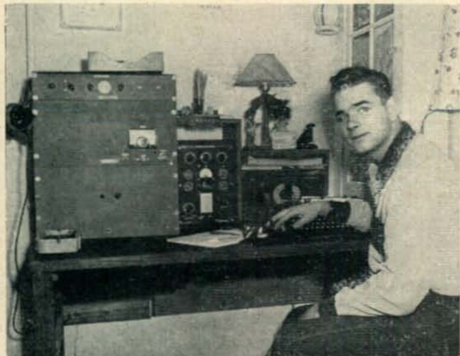
Johnny McGuire, who works for Uncle Sam's Navy, and his Novice station, WN3VAZ. His transmitter is a Harvey-Wells TBS 50C, and the receiver is an S-38B. The rack on the left contains a 10-11 meter converter, an oscilloscope, and the transmitter power supply. Johnny may be overseas when you see this picture.
