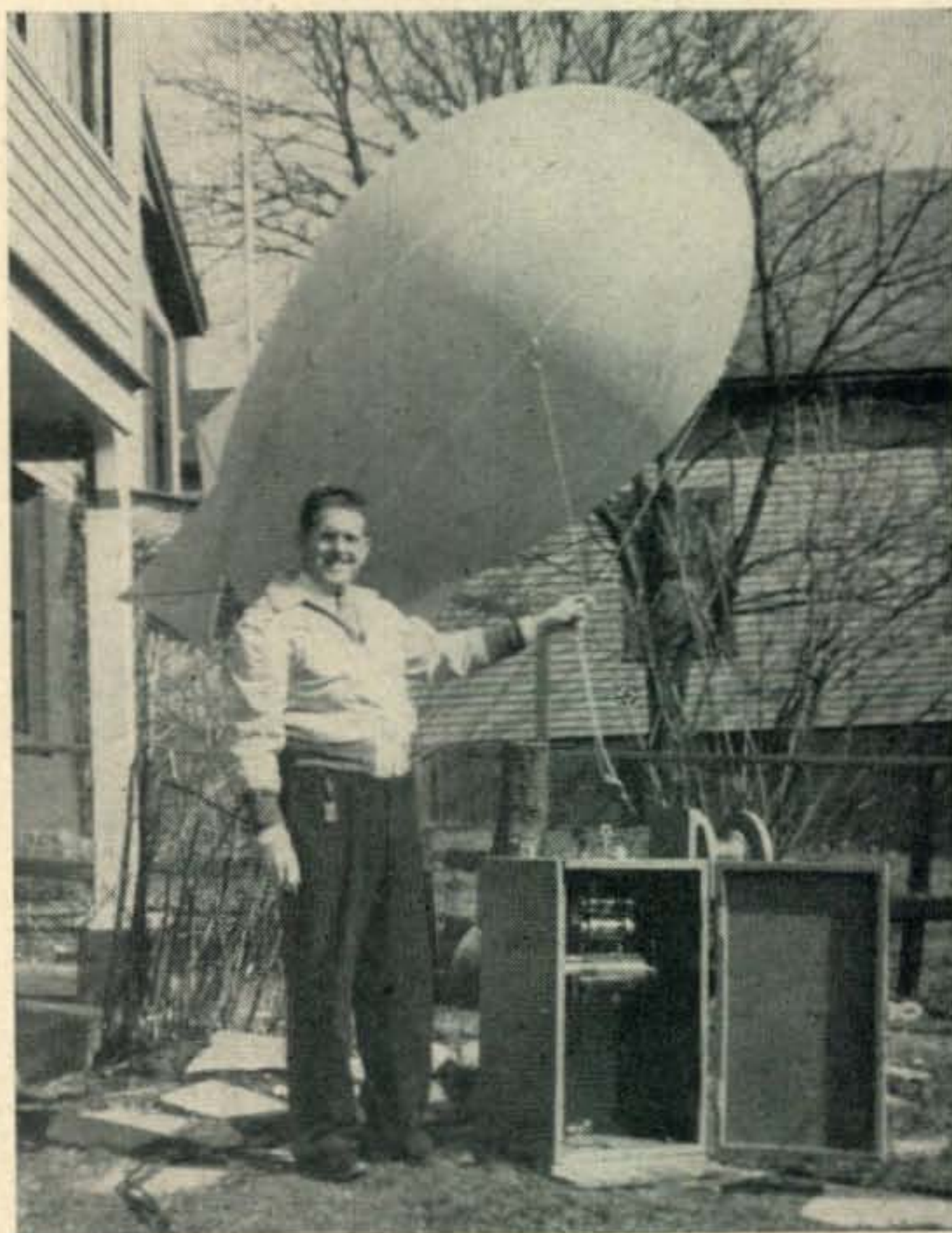
The WIBB KYTOON Antenna has helped to put Stew Perrys' 160-meter signal over with a little more ZIP! (Weather permitting). Stew is seen here in the act of launching the KYTOON which ascends to a height of 260 feet. The antenna tuning unit is contained in the watertight box and is fed from operating position by co-ax.
