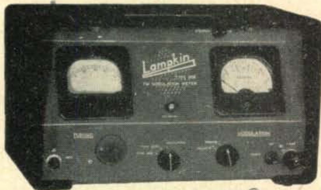
Type 205 FM Modulation Meter. Indicates peak modulation deviation 0-25 kc, either side of carrier. Tunable, 25 to 200 MC. Meets FCC mobile specs. Weight 12 lbs. Width 12". Price $240.00.
