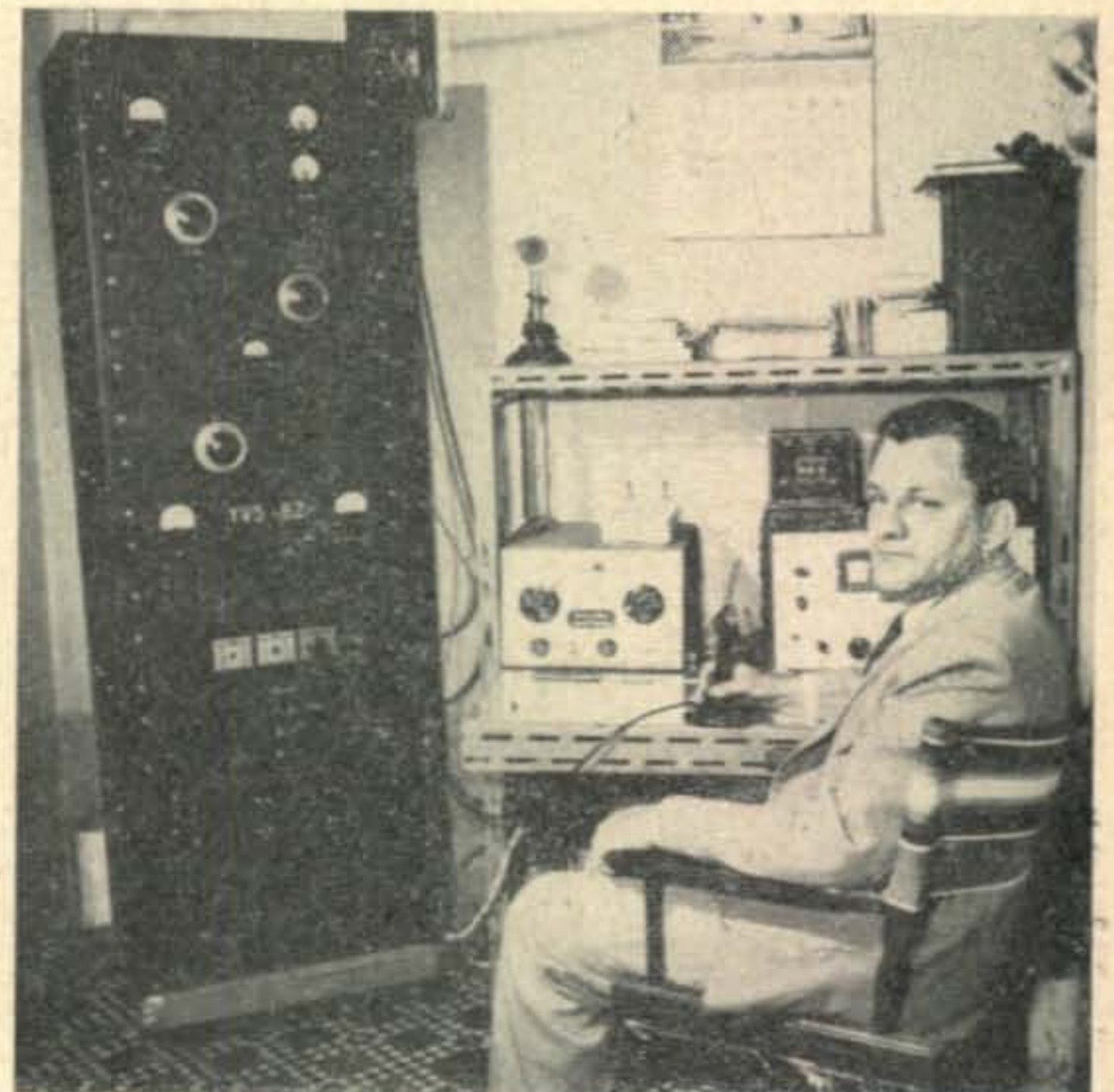
EA4CM attained a score of 88,862 on all bands. His equipment, which is totally home constructed, consists of a 150-watt transmitter with an 813 final, and a double-conversion 16-tube receiver. For antennas he uses a folded dipole on 7 and 21 Mc., and a three-element rotary beam for 14 Mc. . . . YV5BZ scored 61,944 on all bands. Rig winds up with a pair of 813's with 500 watts input. Receiver is an HQ-129X. A 3-element close spaced rotary is used on 20; whip folded dipoles do the job on 10 and 40.
