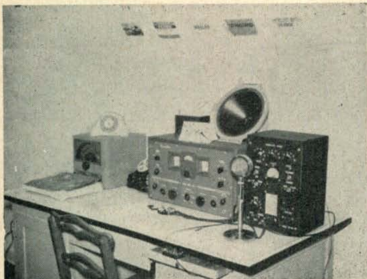
KN2CHS, Scarsdale, N.Y. The first Novice station to report successful DX work on the 21-Mc Novice band. Using a 7-Mc antenna, Dave Smith, the operator, worked five DX countries, including the extremely rare ZD9AA, with fifty watts input. Details in text.
