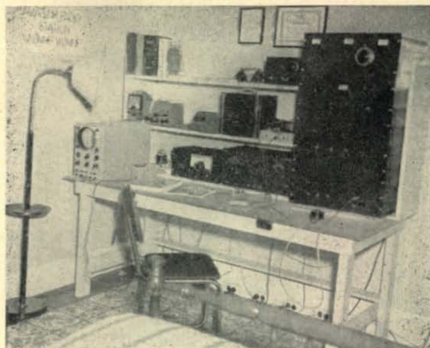
146-Mc. station, WNØMNP, operated by Ronald Tipton, 16, in Kansas City, Missouri. The transmitter at the right uses a pair of 815's in the final. Receiving is done with an S-76 receiver and a home-built converter. Also visible on the left side of the bench are cathode-ray oscilloscope, vacuum-tube voltmeter, signal generator and grid-dip oscillator. Ronald's latest acquisition is a fifty-foot tower upon which he is erecting a rotary beam.
