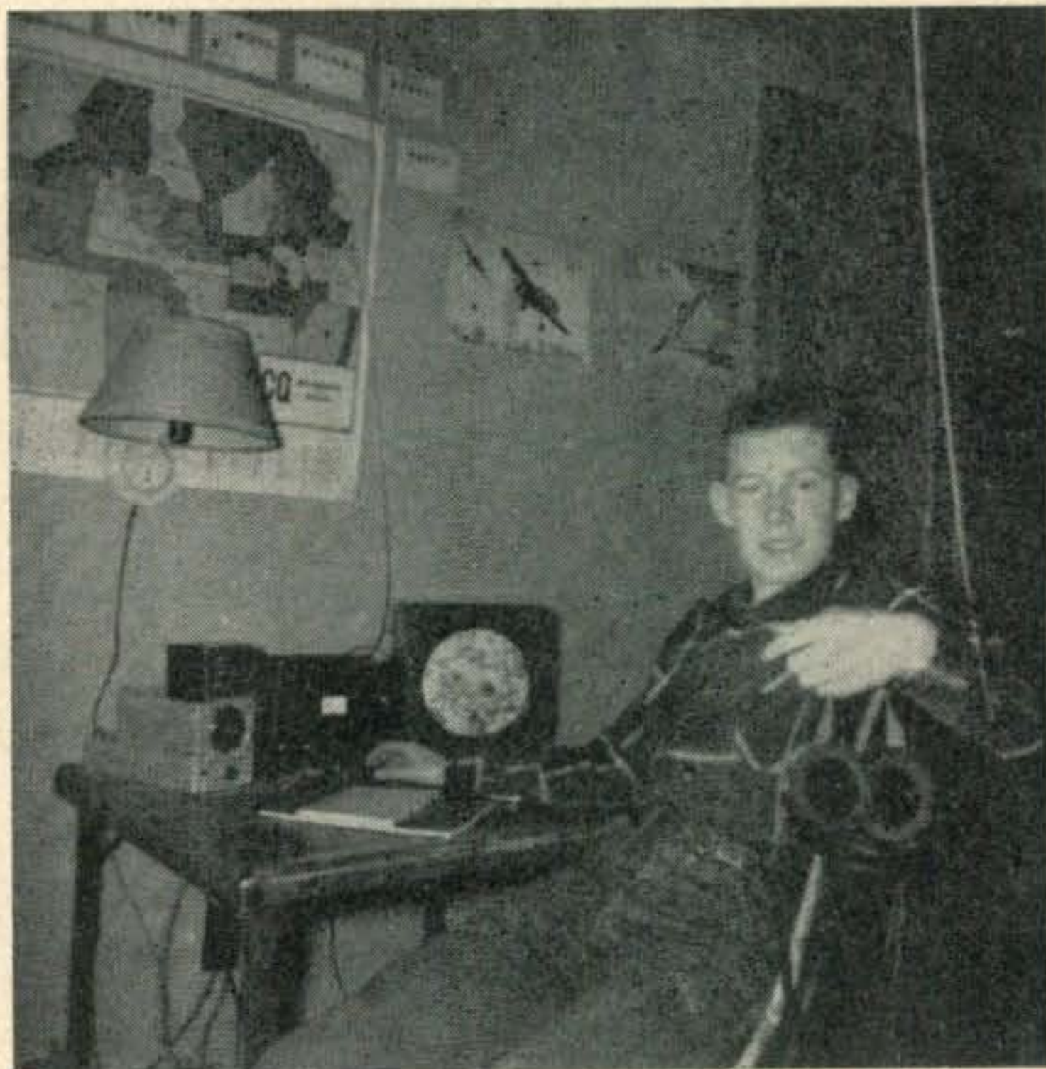
Ward Helms, 14, at the key of WN7SXM. His transmitter runs fifteen watts to a 6V6 and his receiver is a BC-454. Best DX on 3.7 Mc. is 1000 miles.
