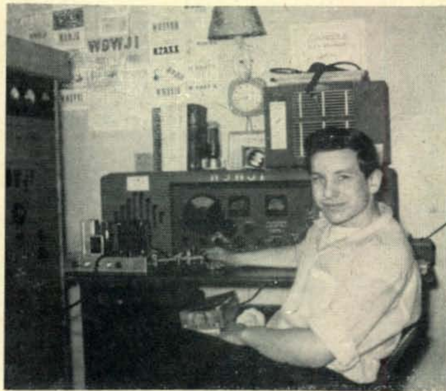
Tom Hamel, 16, who was waiting for his General Class license when this picture was taken, and his attractive station W9WJI, Chicago. The rack to the left must be for future expansion, because his rig is a 6AG7-6L6, with 30 watts input.
