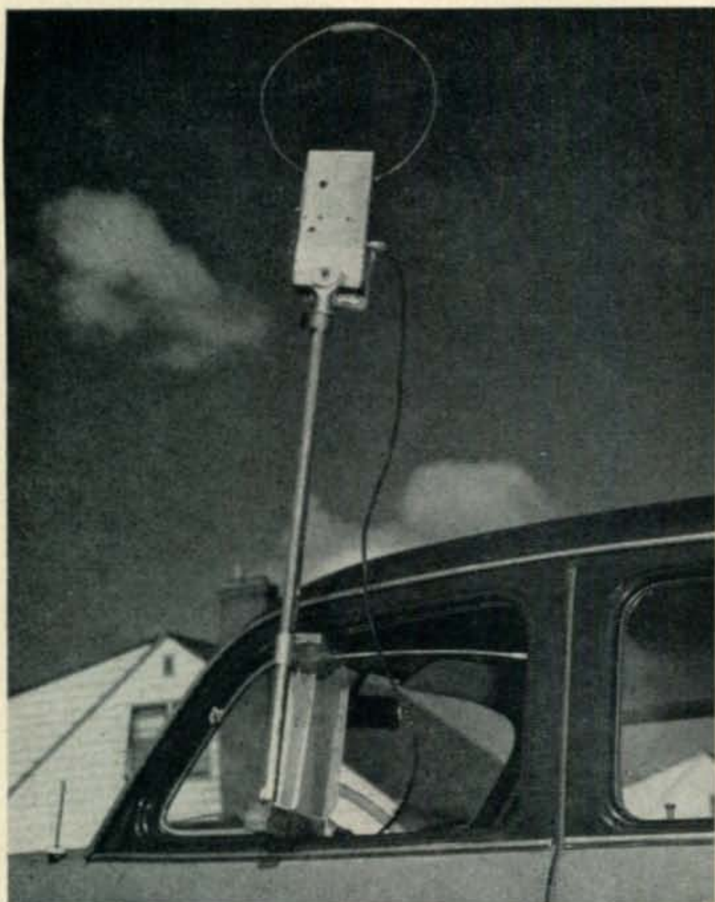
This loop, built into the box from a BC610 plug-in exciter unit, utilizes the type of window-frame mounting which is described in the text. The upright piece was salvaged from an old sun-lamp.
