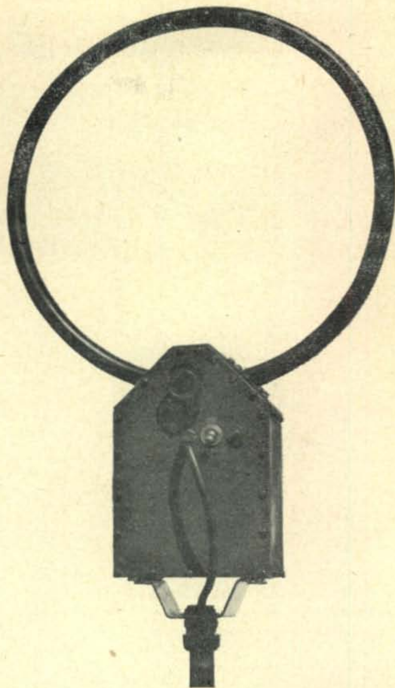
An exterior view of the r-f amplifier loop. The s.p.s.t. switch is in series with the loop filament, and may be turned off when in close proximity with the hidden transmitter.
