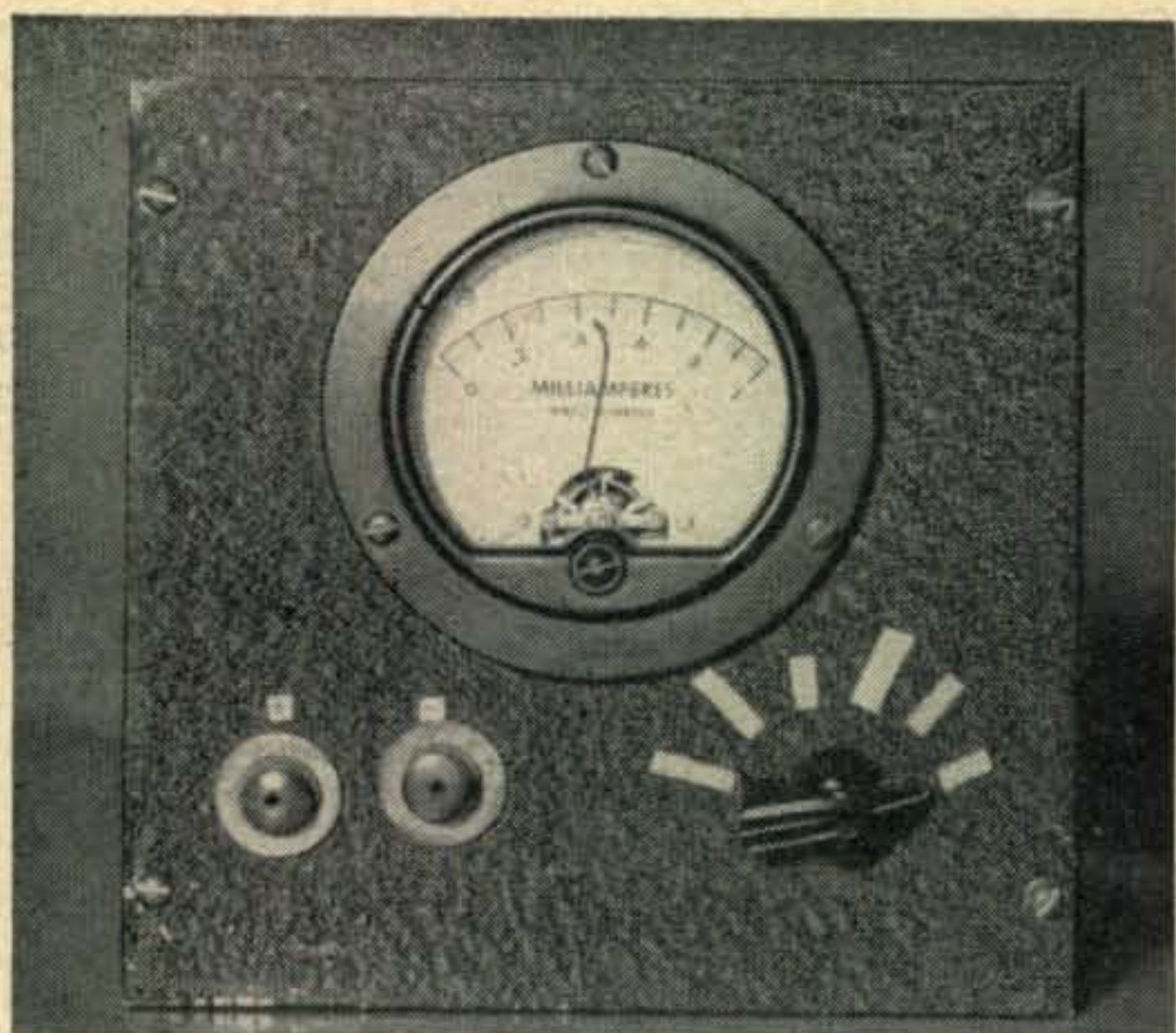
Learning a lesson the "hard way." No fuse— now no meter!
