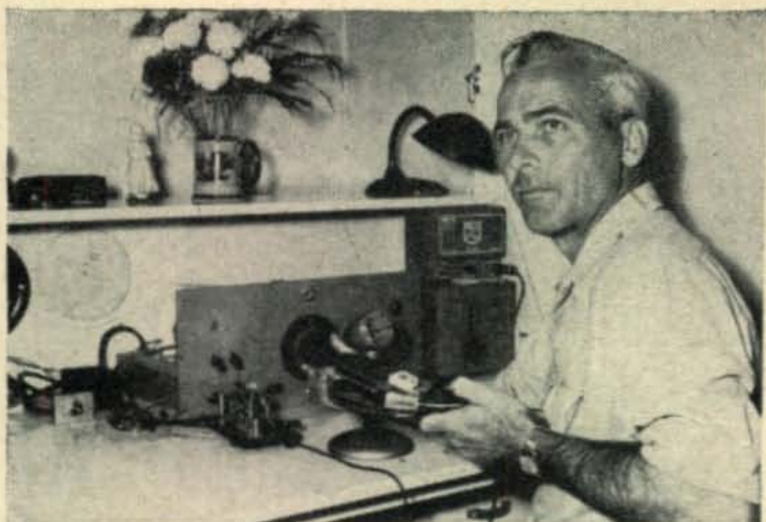
W6BAX, "Opie" Taylor, San Carlos, Calif. needs no introduction. Licensed in 1927 Opie was one of the top pre-war DX men. The rig, remotely controlled from this position in the kitchen, runs 800 watts to PP 4/125A's assisted by a three element rotary beam. W6BAX sticks to 14 Mc. and his present CW score is 222 countries. The homebrew receiver pictured above has since been replaced with a Collins 75A2. (Photo: North California DX Bulletin)
