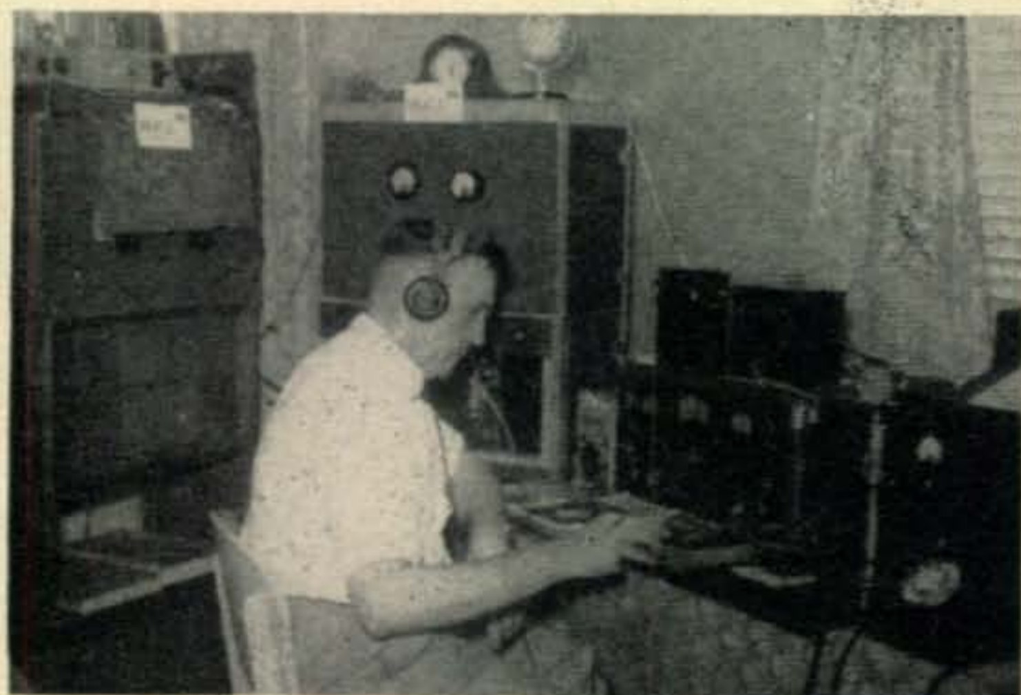
VK4FJ, Roy Baxter, Brisbane, Australia is the man behind one of the most consistent signals from "down under." Roy runs 75 watts to PP807's on 28, 21 and 14 Mc. and 100 watts to an 813 on 7 Mc. The country total at VK4FJ is 207; AC4NC QSL is awaited for WAZ.
