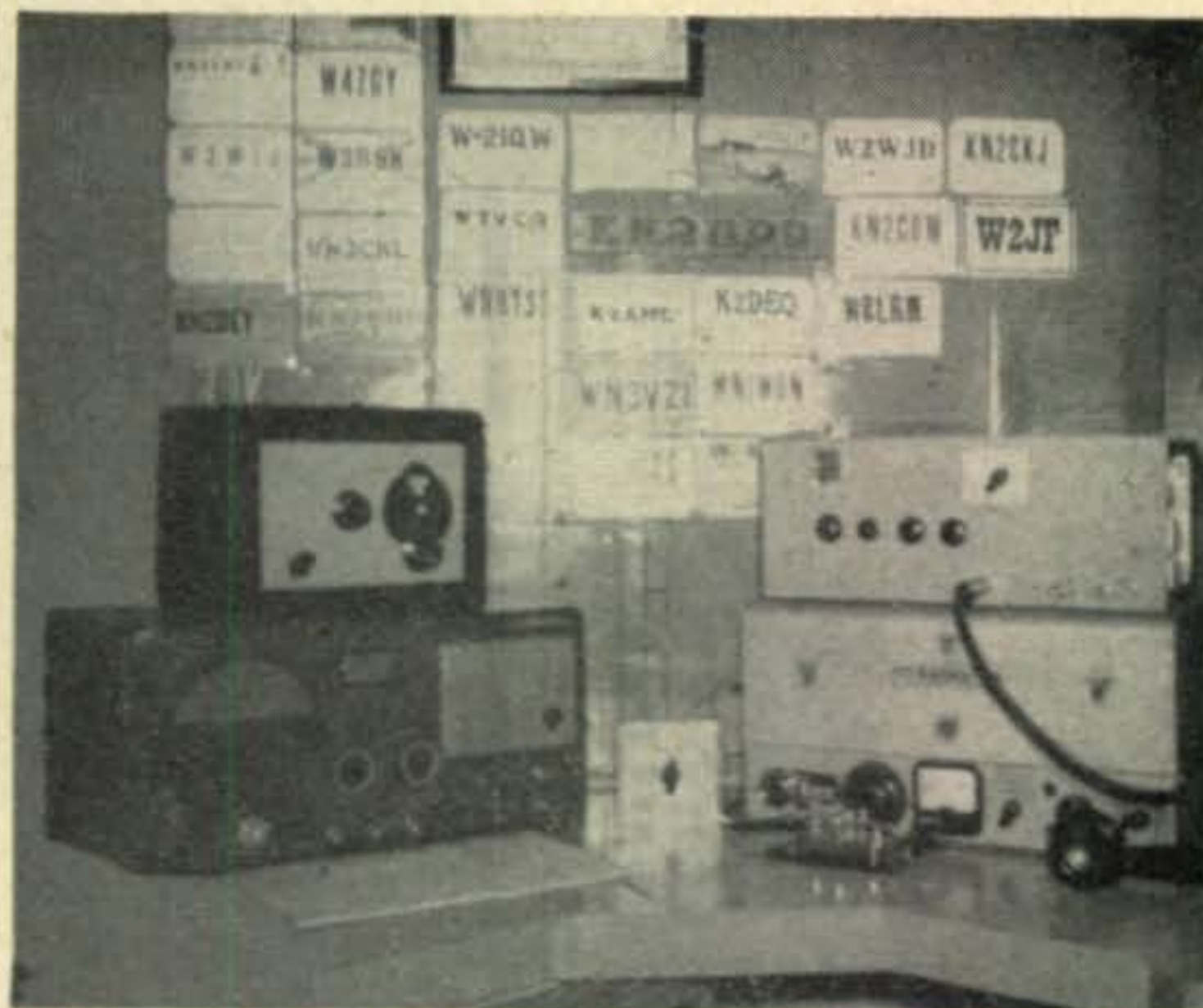
KN2DPQ, Pleasantville, N.J. Transmitter is a TR75 and receiver is an S-40A. Unit on top of receiver is a 146-Mc converter. The one on top of the transmitter is a converted BC-625 (522) transmitter for 146 Mc.
