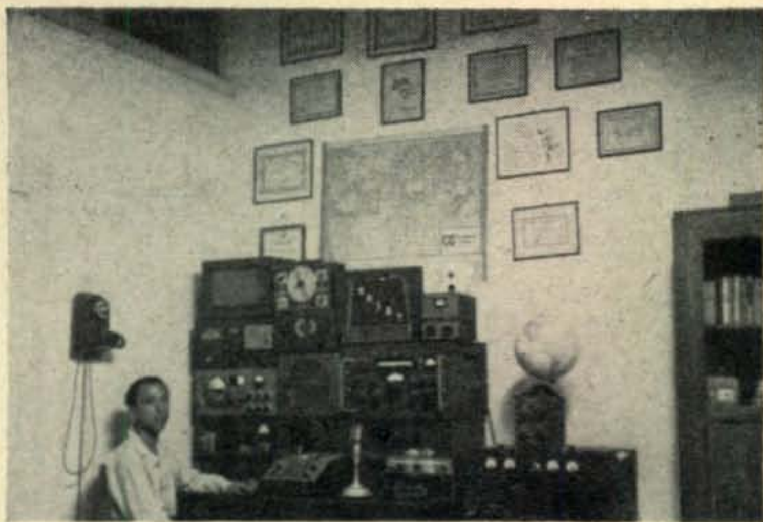
HRIAT, Oscar Trochez, of Tegucigalpa, Honduras is active on all bands Phone and CW. Set-up runs a Viking VFO-6L6-807 which pushes an 813 to 150 watts. Oscar, who is now acting as HR QSL Mgr. wants it known that he is on every day at the following times: 1900/2000 GMT on 21 Mc., 2000/2100 GMT on 14 Mc. and from 0400/0600 GMT on 7 or 3.5 Mc. HRIAT went on the air in 1947 and has worked 105 countries and about 2000 W's.
