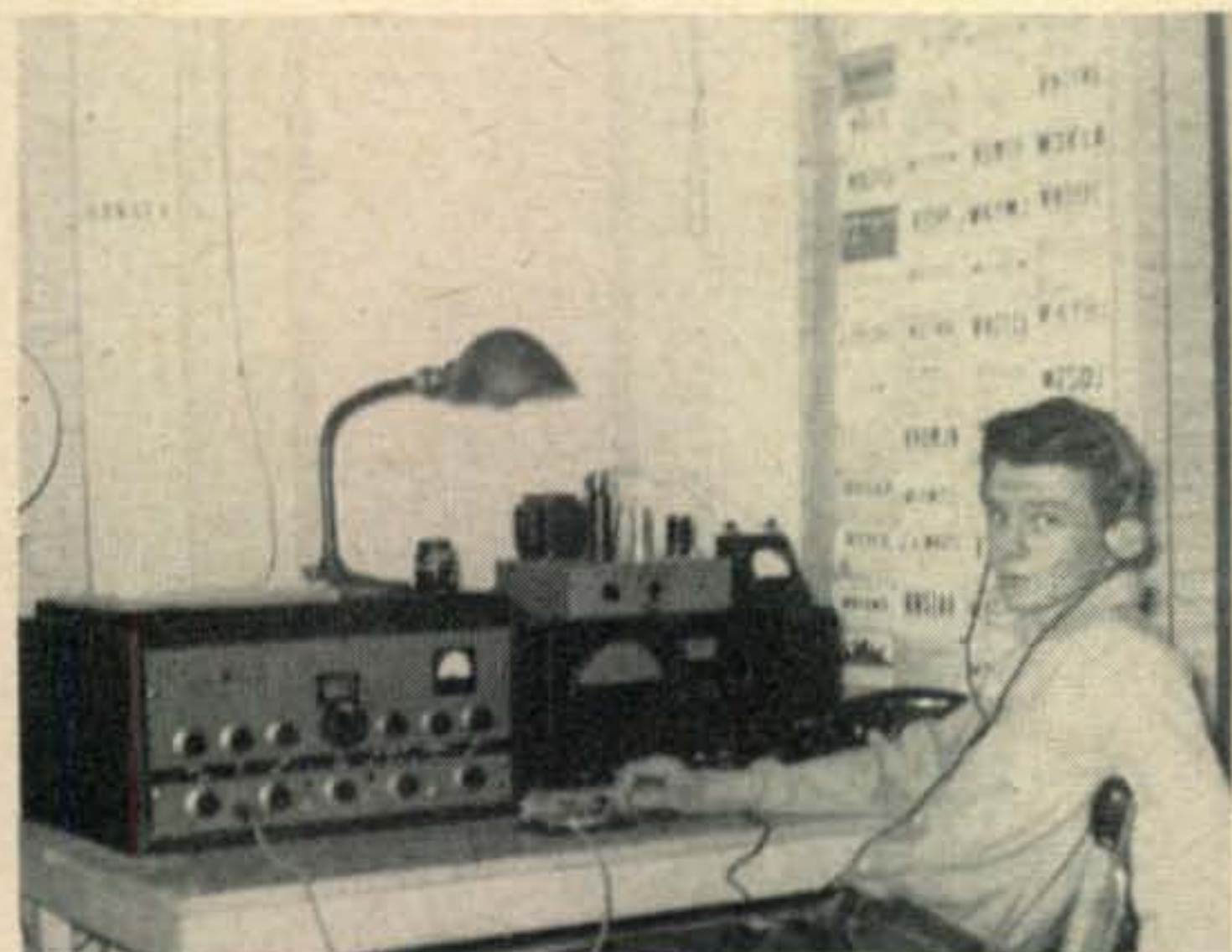
With the equipment shown in this picture, Ralston, WN5ZNN, has worked 42 states. Maximum power used is 70 watts. Antennas are ground planes for 40 and 15 meters, and a doublet for 80 meters.
