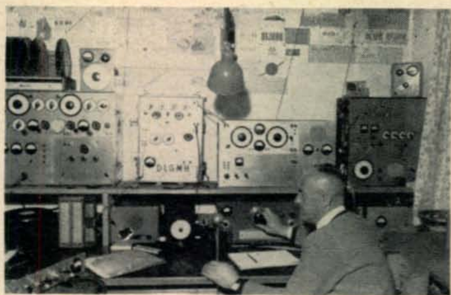
DL6MH listening for the weak ones on 2-meters. The receiver combination includes a Wallman in an HRO. The transmitter is 100 watts input.
