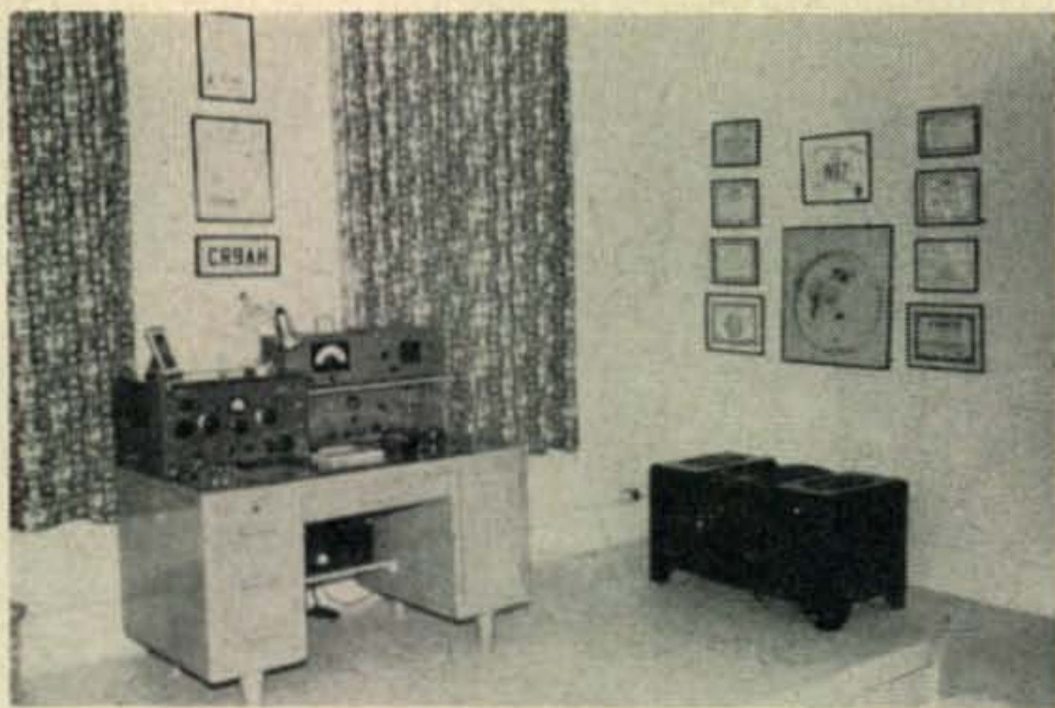
The neat set-up of CR9AH, John Alvares, Macao. Two 807's in parallel are used and modulated by and 829B. The antenna is a dipole fed with 73-ohm co-ax, fifty feet above a two-story building. All gear is home-built.
