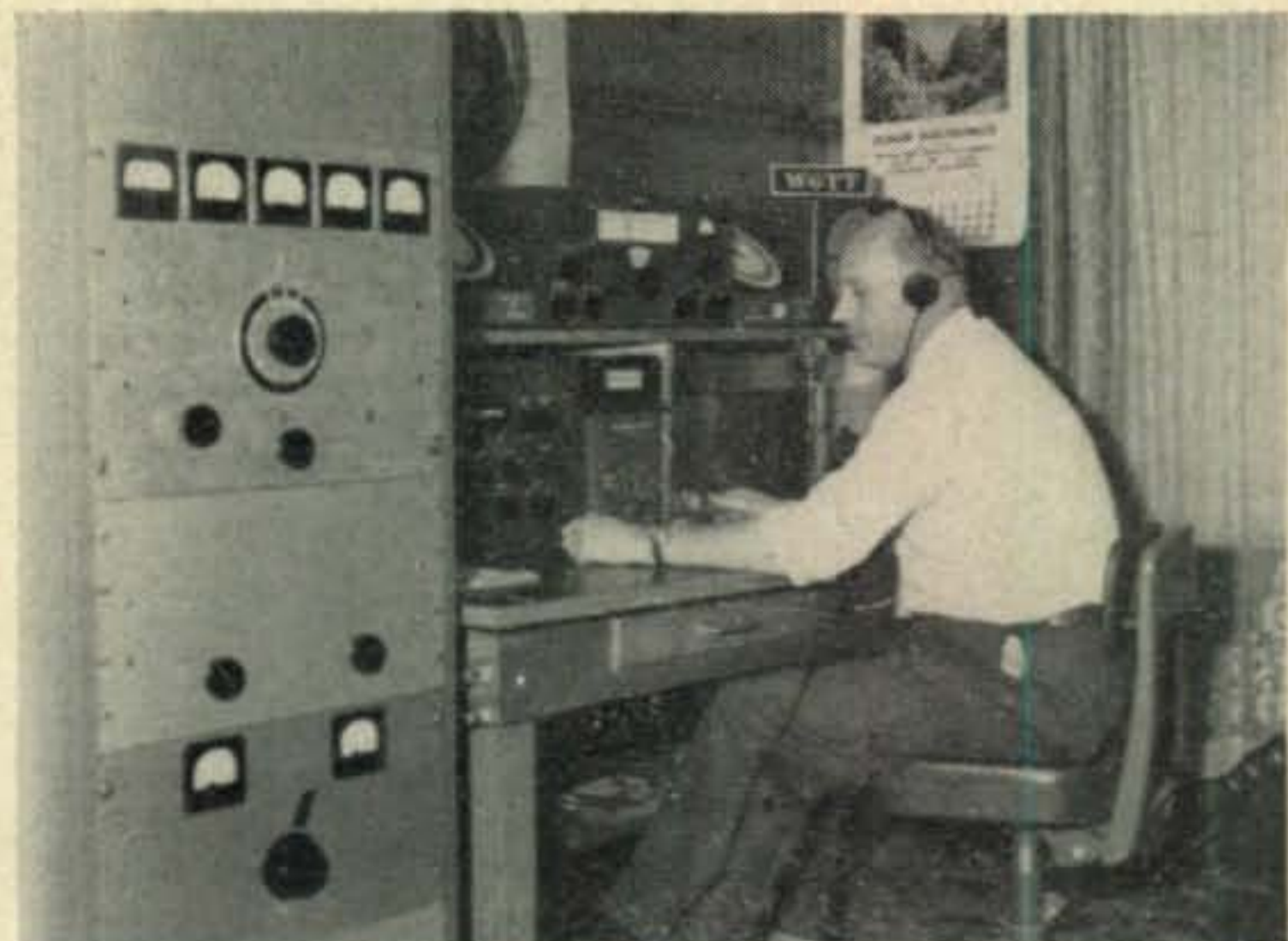
Ye Olde DX'er, Elvin Feige, W6TT of Oakland, Calif., needs no introduction. The rig consists of a Collins 310B1 exciter driving a pair of 4-250A's on phone and CW. Single sideband is also used. Receiving gear consists of an 75A-3, RME DB23 converter and sideband slicer. 3-element beams are used on 14 and 28 Mc. while 3.5 and 7 Mc. is taken care of by half-wave dipoles. W6TT's score stands at 230, with 225 confirmed, and 142 on A3. Photo courtesy of No. Calif. DX Bulletin.
