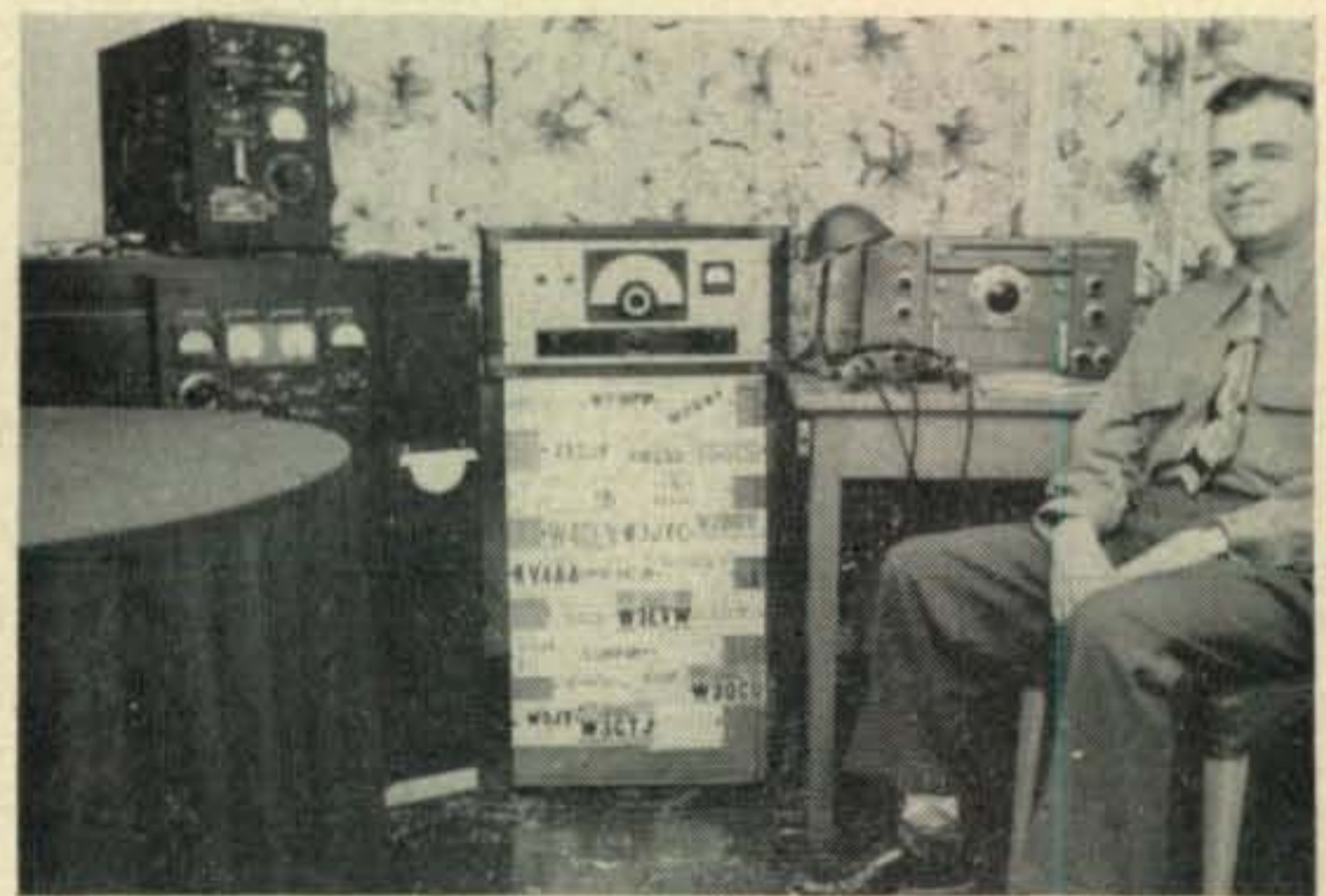
The operating position of KR6AA in Okinawa. Doc Westervelt, W4VE, uses the small 50-watt band switching rig, which was his complete transmitter at KA9AA and KA2AA, to drive the 610 at 400 to 500 watts. The 7 Mc. band should now be available for use by KR and KA stations and Doc plans plenty of activity there. The antenna is a 700-foot long wire.
