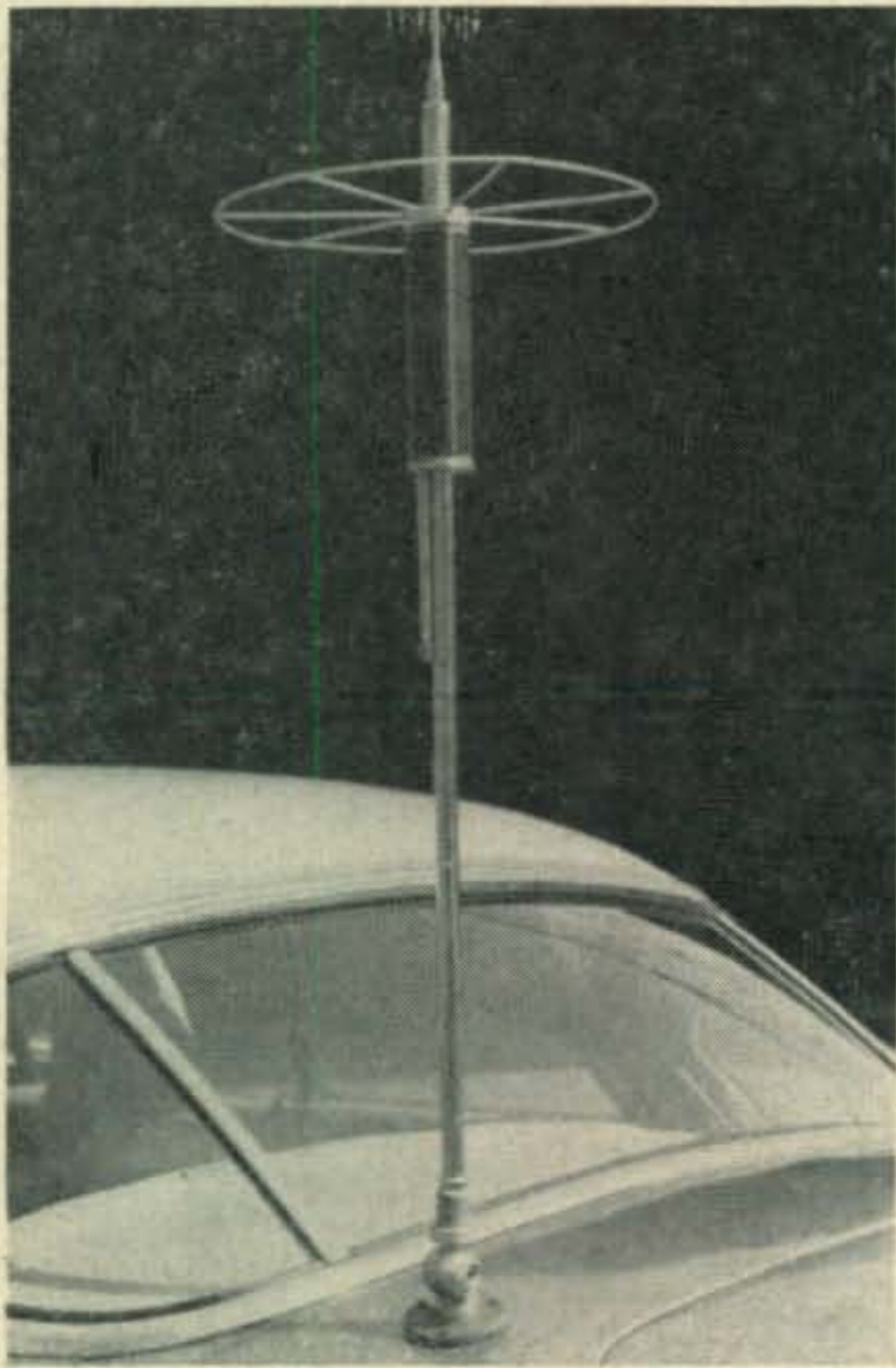
An example of near-center loading with a "capacity hat" and single-band fine tuning is this W3GH "Green Hornet" mobile antenna. See text for details.
