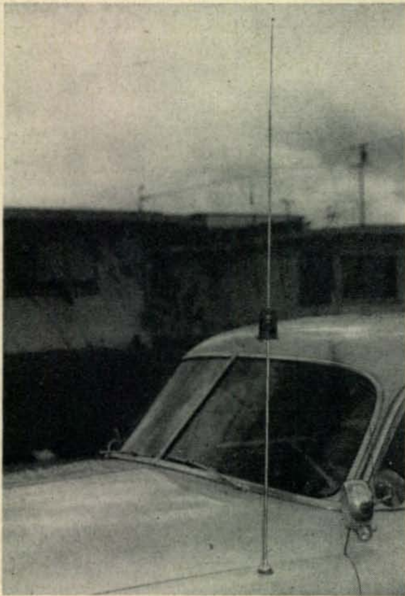
The "VS Baby" is a very compact center loaded antenna for mounting on the cowl or fender. A plastic housing protects the loading coil.
