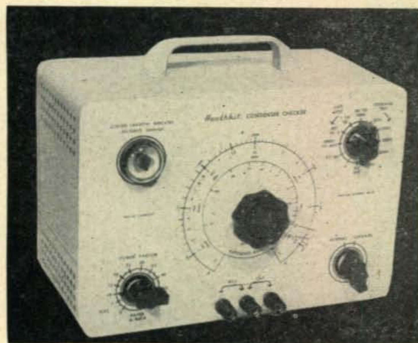
A useful item around the Ham shack is a condenser checker. The Heathkit model can also be used as an ohmmeter in a pinch.
