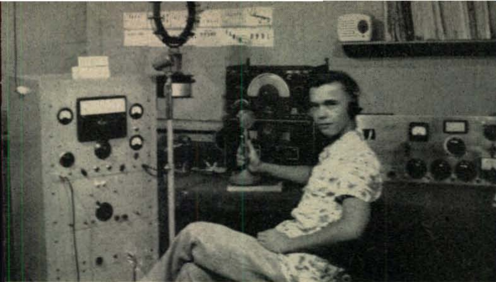
FK8AL, Noumea, New Caledonia, op Jean Garbe, may be seen above. FK8AL may be found every weekend on 14 Mc. between 0300 and 0600 GMT. Jean is also active on 3.5, 7 and 28 Mc. Parallel 807's are run on CW and phone. Receiver is a BC-342. This station is also operated by "brother" Robert Garbe under the call of FK8AH.
