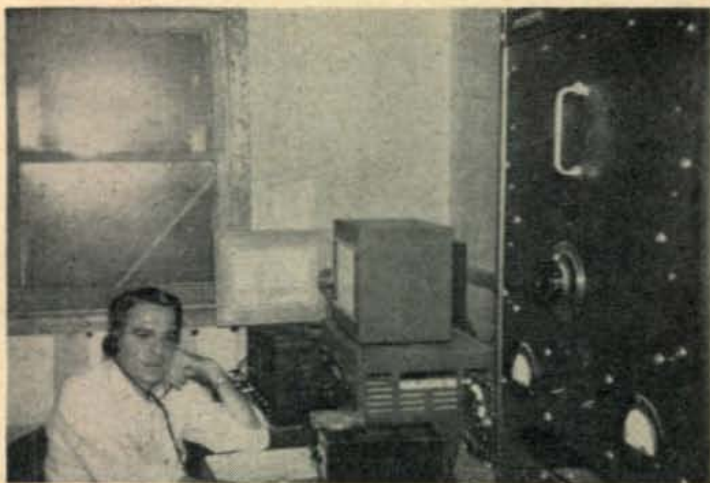
W5MIS, Tom Perry, Tulsa, Okla. runs a pair of 813's to a 3 element beam. The exciter is a Collins 310B. Very active in the DX field Tom's country total is in the 240's. (Photo: W5FFW.)
