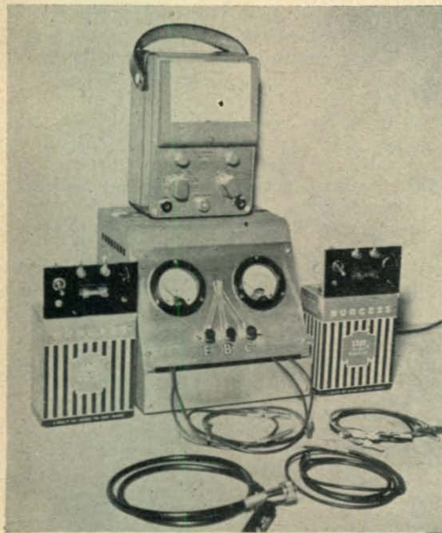
The author's test setup for transistor experiments. Low current fuses protect the transistor.
