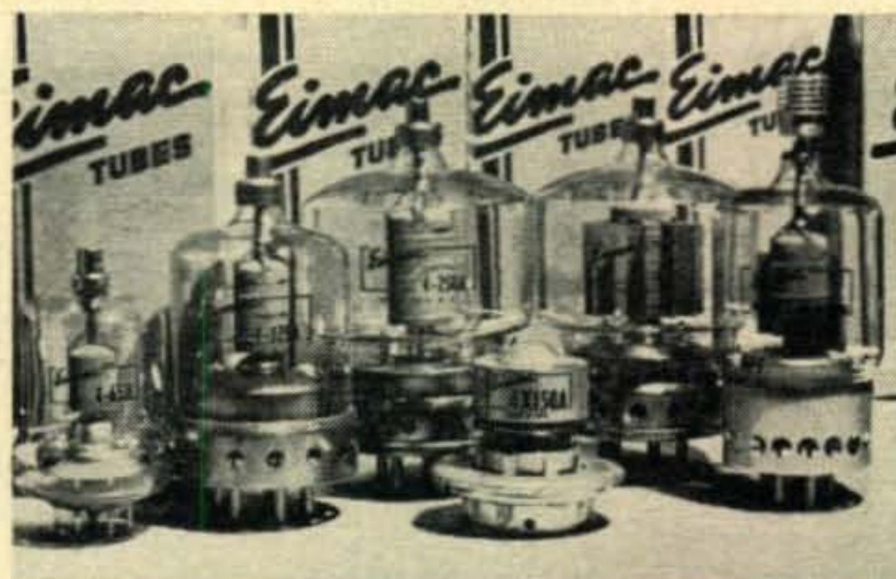
The Big Six of Amateur Radio: 4-65A, 4-125A, 4-250A, 4-400A, 4X150A, 4E27A
