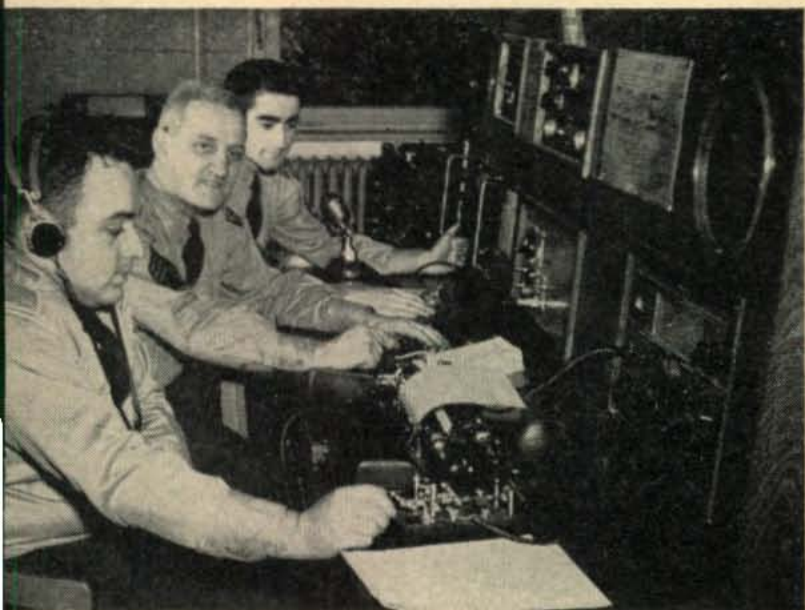
A view of MARS Station OE13USA, located in Camp Roeder, Salzburg, Austria. Operators: (l to r) Marty Goen, K21XD, M/Sgt "Mac" McKenna and Doug Murray, W6HVN. OE13USA handles a large amount of phone patch traffic and other traffic. Over 700 QSO's were handled during the Xmas season. A BC-610 runs 500 watts on phone and CW and a remotely operated KW to a pair of 833's. Receivers: a Collins 51-J and a revised 75-A-2. Three element beams are mounted on an eighty foot tower. OE13USA may be found on or near 14180 or 14315 from 0700 GMT to 1700 GMT and then swings down to about 14035 for CW. Photo: U. S. Army.
