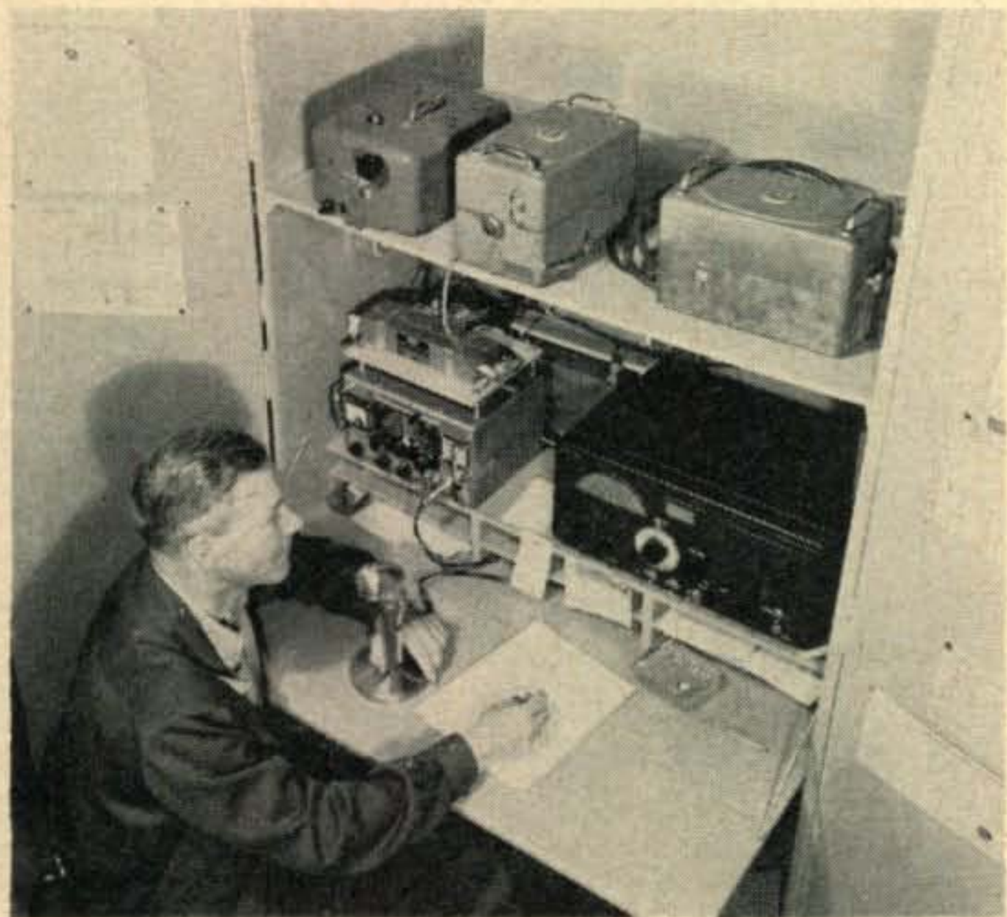
Herbert Clark, Jr. contacts a mobile unit from W9FKV net control, which controls five CD mobile units. A Motorola P-69-17A mobile receiver monitors the Chicago CD net frequency, and a spare T-69-20A transmitter is available when needed. (photo courtesy Motorola)
