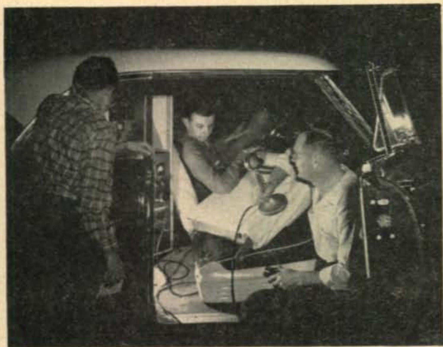
W5ANQ/M, with Collins 75A1 and Viking II rack-mounted on rear-seat supports. Installation includes a separate dash-mounted 6v. station.
