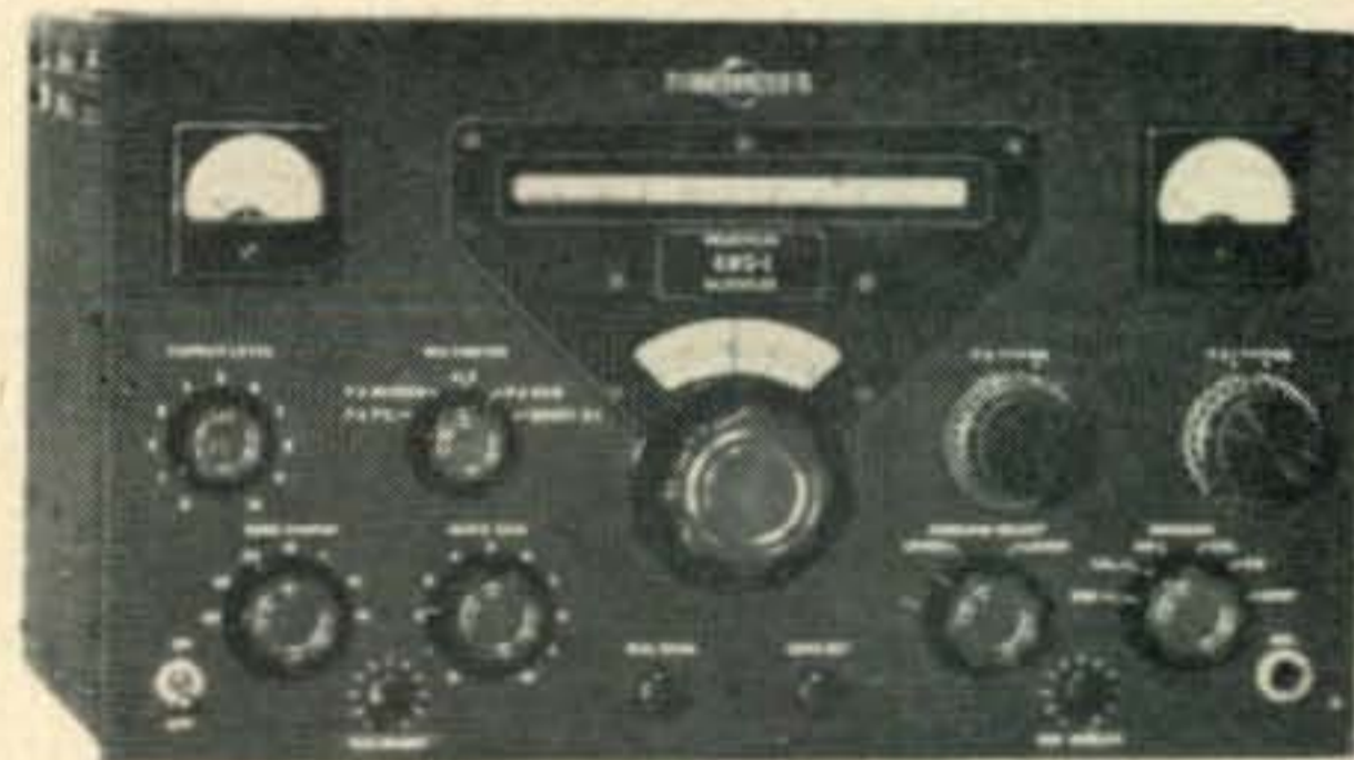
The exciter and power amplifier of Collins KWS-1 transmitter are housed in small, compact receiver-size cabinet.
