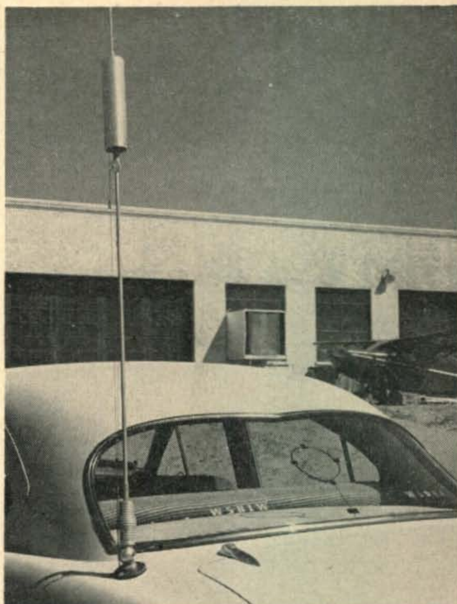
Coil in place. Note dial cord for remote tuning, and field strength loop in rear window.
