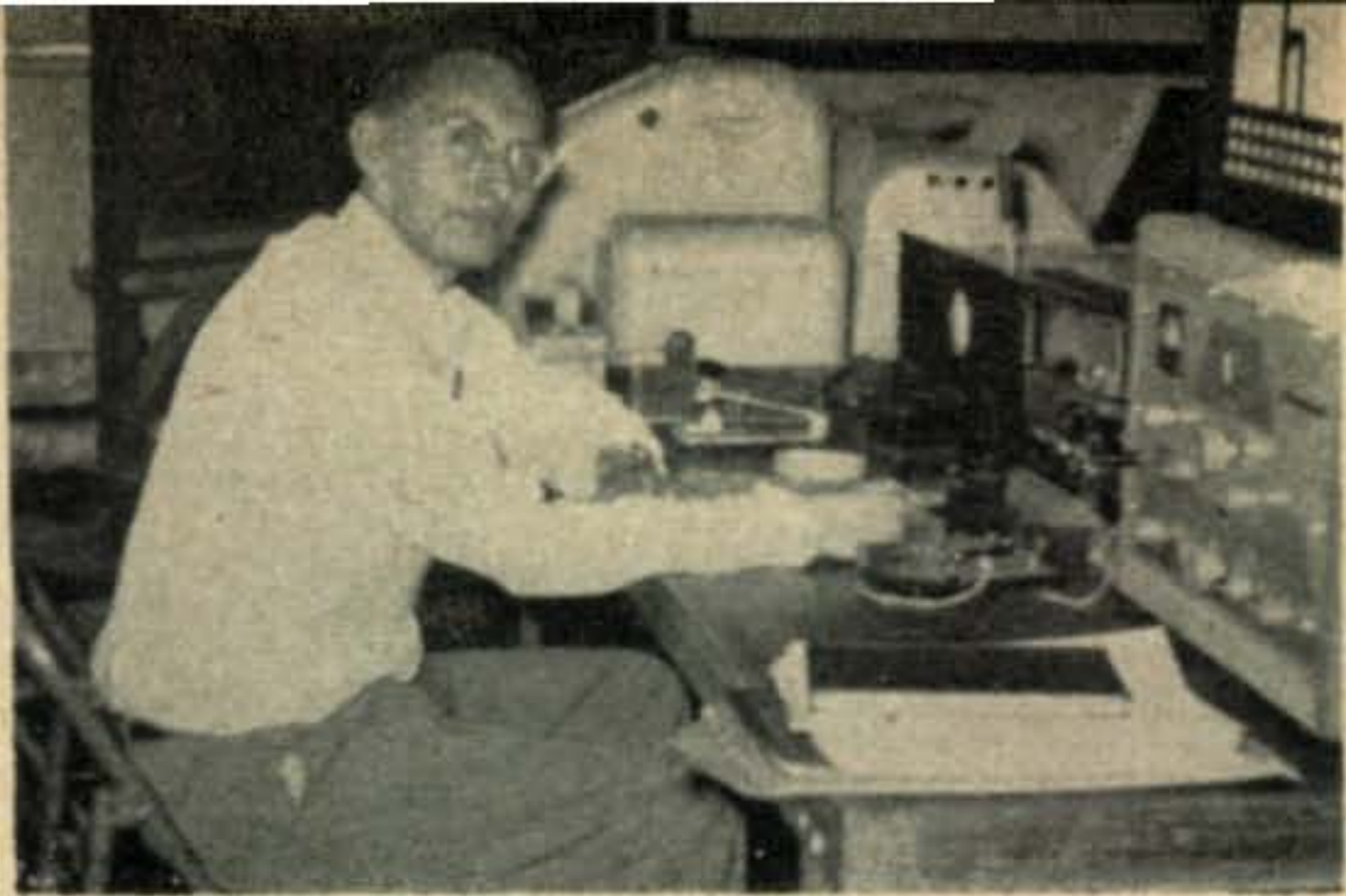
Bob Unsworth, W6MTJ, at the operating position of W6AEE/6 at the Pacific Division ARRL Convention May 21, 1955. That's a DX-100 Heath Kit transmitter, modified for FSK, at the far right end of the operating table. The receiver is an SX-96. The terminal unit is W6AEE, described in December 1952 CQ. Photo is by W6ZNU.
