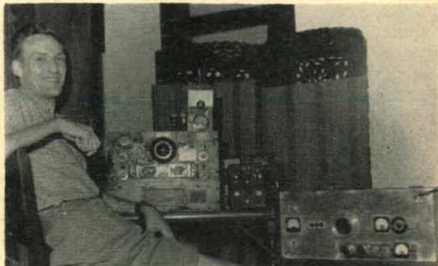
4S7PT, manned by Pete Rudd, Colombo, Ceylon, runs 45 watts to an 807. Rx is an HRO and the skywire a folded dipole. Pete was D2IX in '47.
