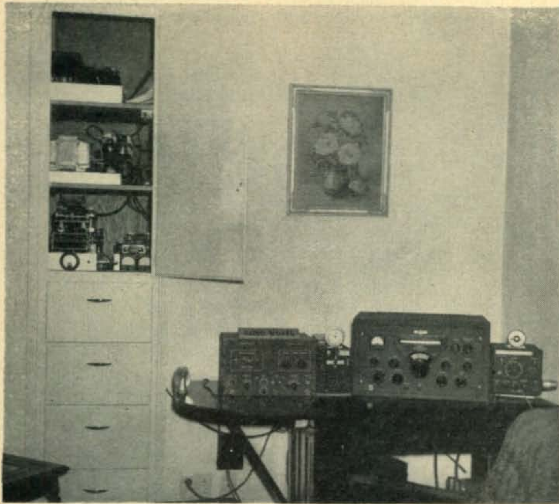
On the air, W6FIS looks like this. This former linen closet, from top to bottom, now houses on the top shelf a 1200-volt power supply for the 837's. A 2,500-volt supply for the 803's is next, while the lower shelf contains the 803 final and the 837 drivers.
