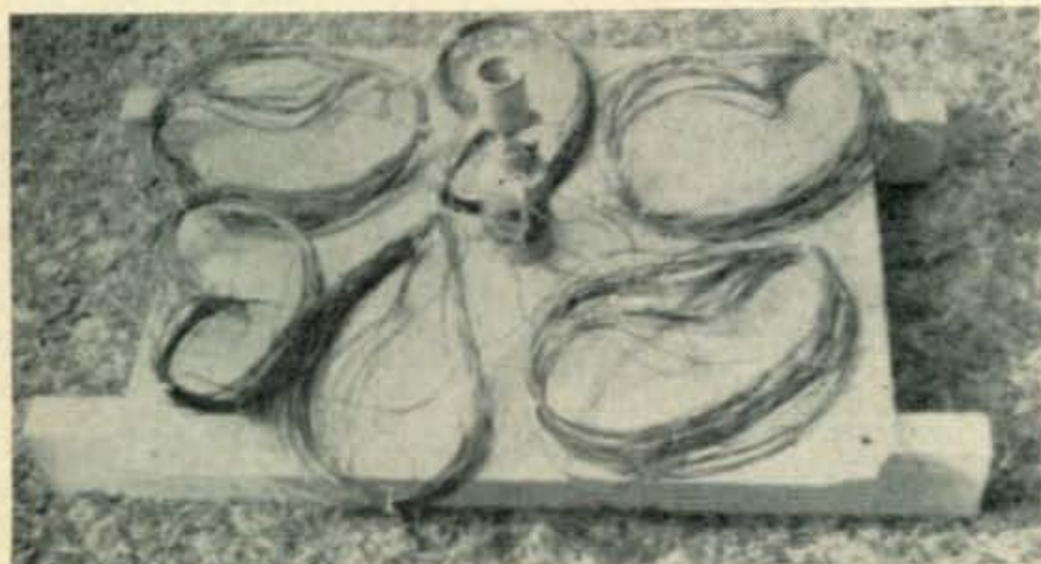
Ground screen, base insulator and frame, with 62 foot radials cut and rolled into coils await hoisting atop garage roof. Ground screen is scrap dural 20x24 inches.
