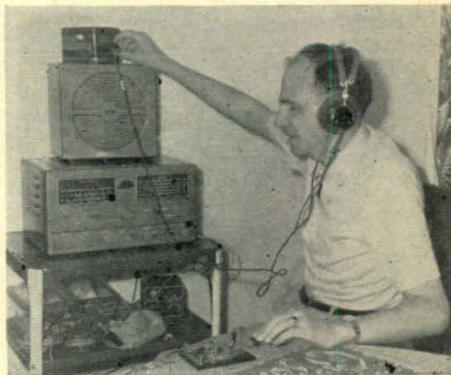
Philip Leonard, KN6MTN, tunes his field strength meter to resonance.
