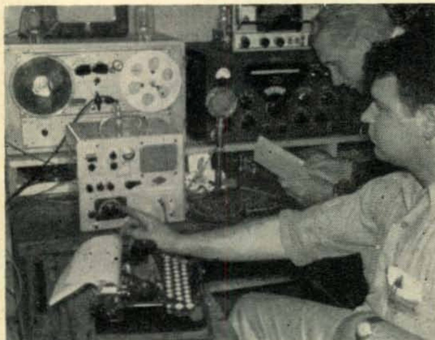
W3ZVK, second highest scorer in Pa. Rig is a Gonset Communicator, antenna a 5-element beam 20 feet high, QTH is 520 feet above sea level.
