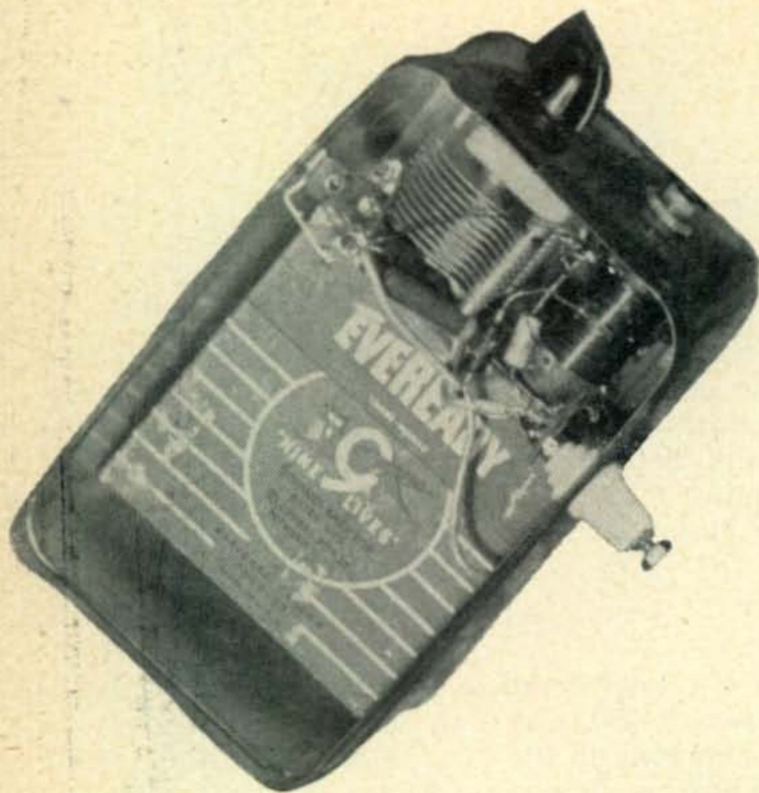
FS Meter, cover removed
