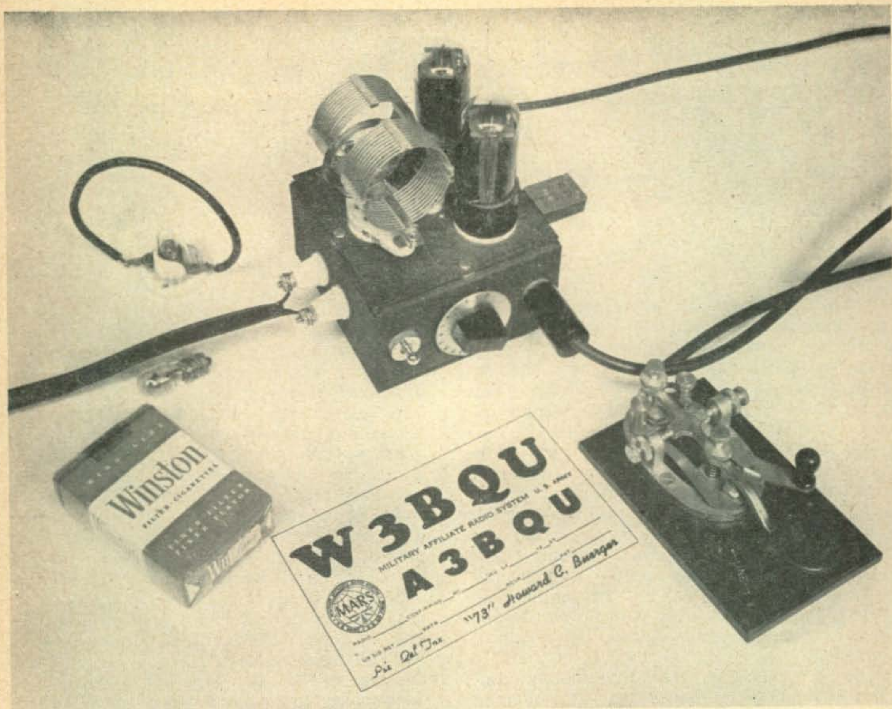
The key, QSL card and cigarette package sort of dwarf the "lil" rig. The neon bulb is used to indicate the maximum xmtr output when placed near the antenna feeder. The wire loop on the pilot bulb makes a useful gadget for checking resonance of plate circuit
