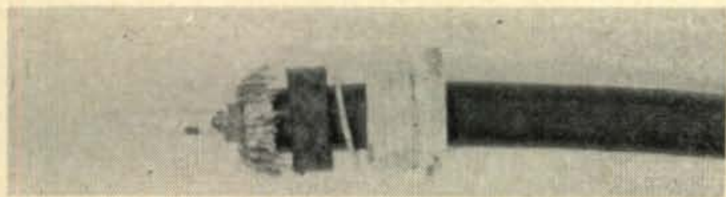
Fig. 2. Before soldering female and male BNC connectors the assembly should look like this.
