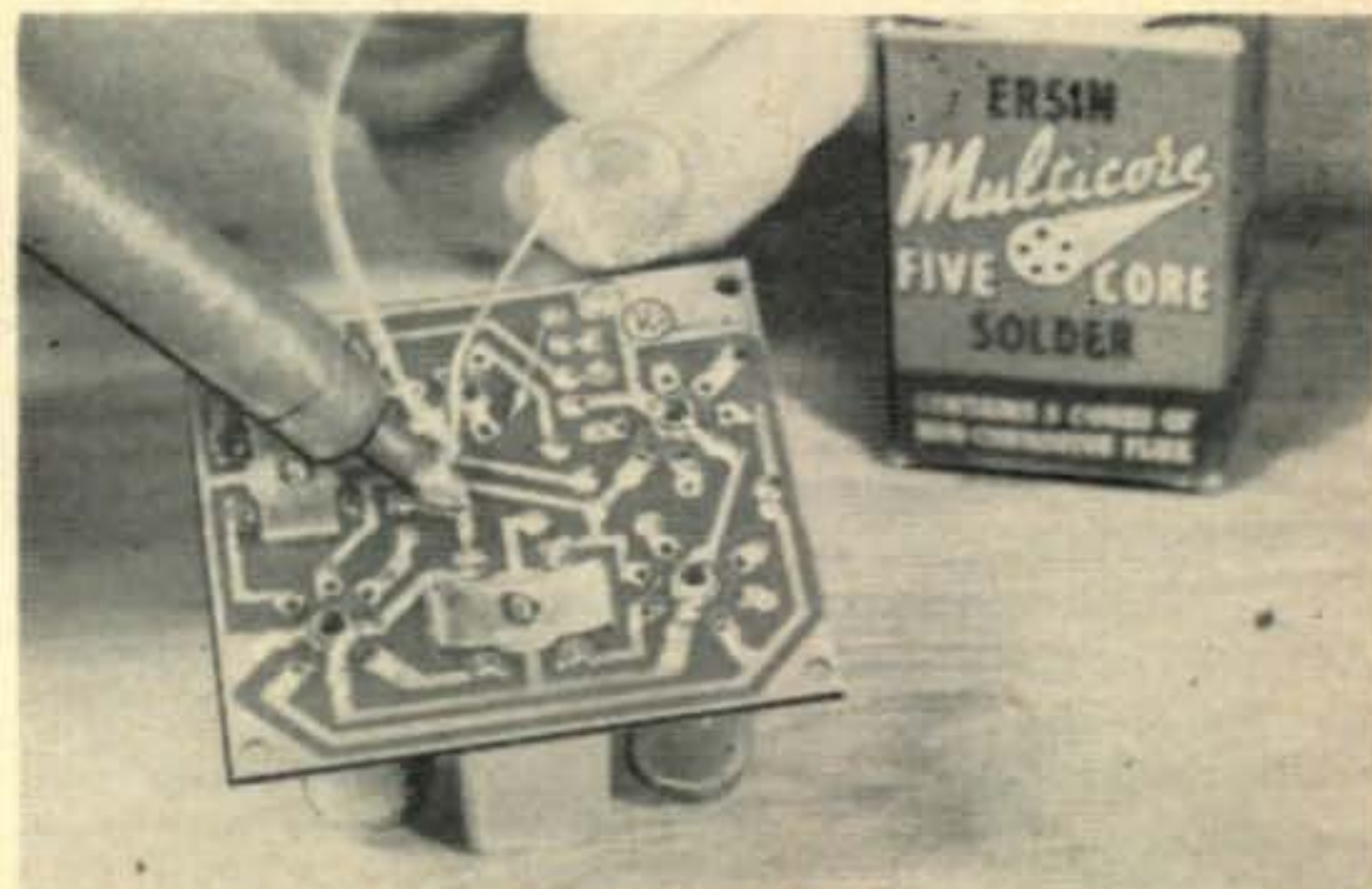
Fig. 14. Soldering Components in Place
