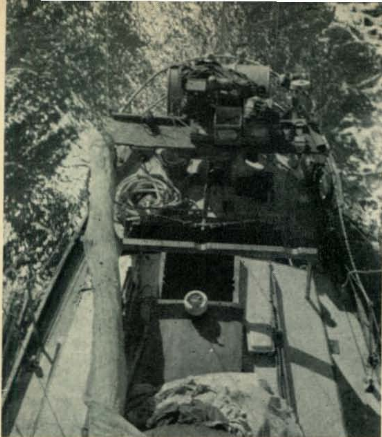
Yasme, looking aft. Note the lashed tiller permitting the boat to "drive herself."
