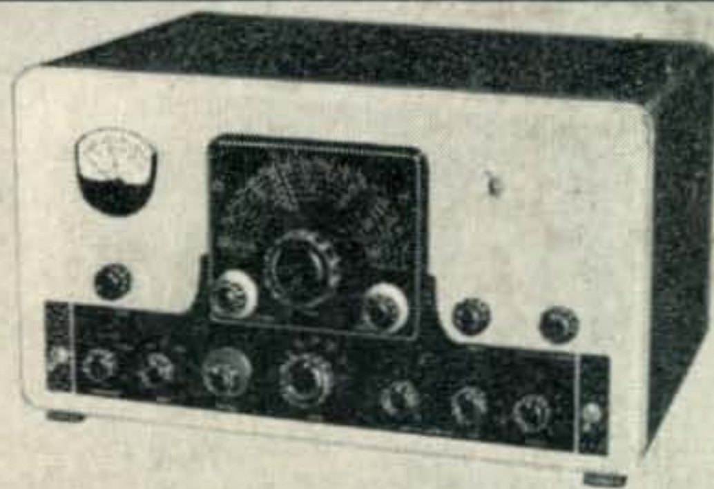
• Viking Valia uses three RCA-6146's in parallel final, two RCA-6146's in p-p class AB 2 modulator.
