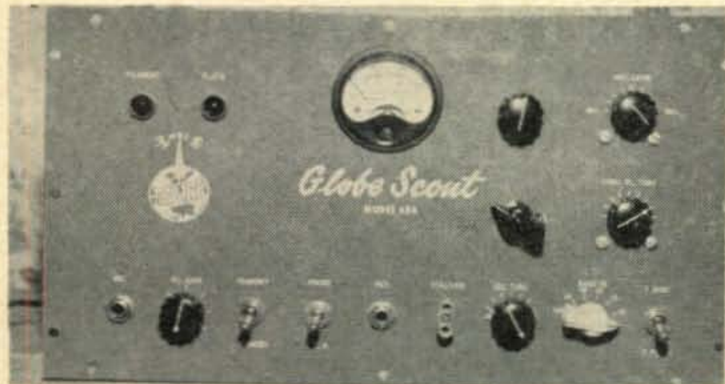
Globe Scout, New controls are the tank circuit and modulated B plus switches for the two meter transmitter and the six meter tuning condenser. Note position of the band-switch.
