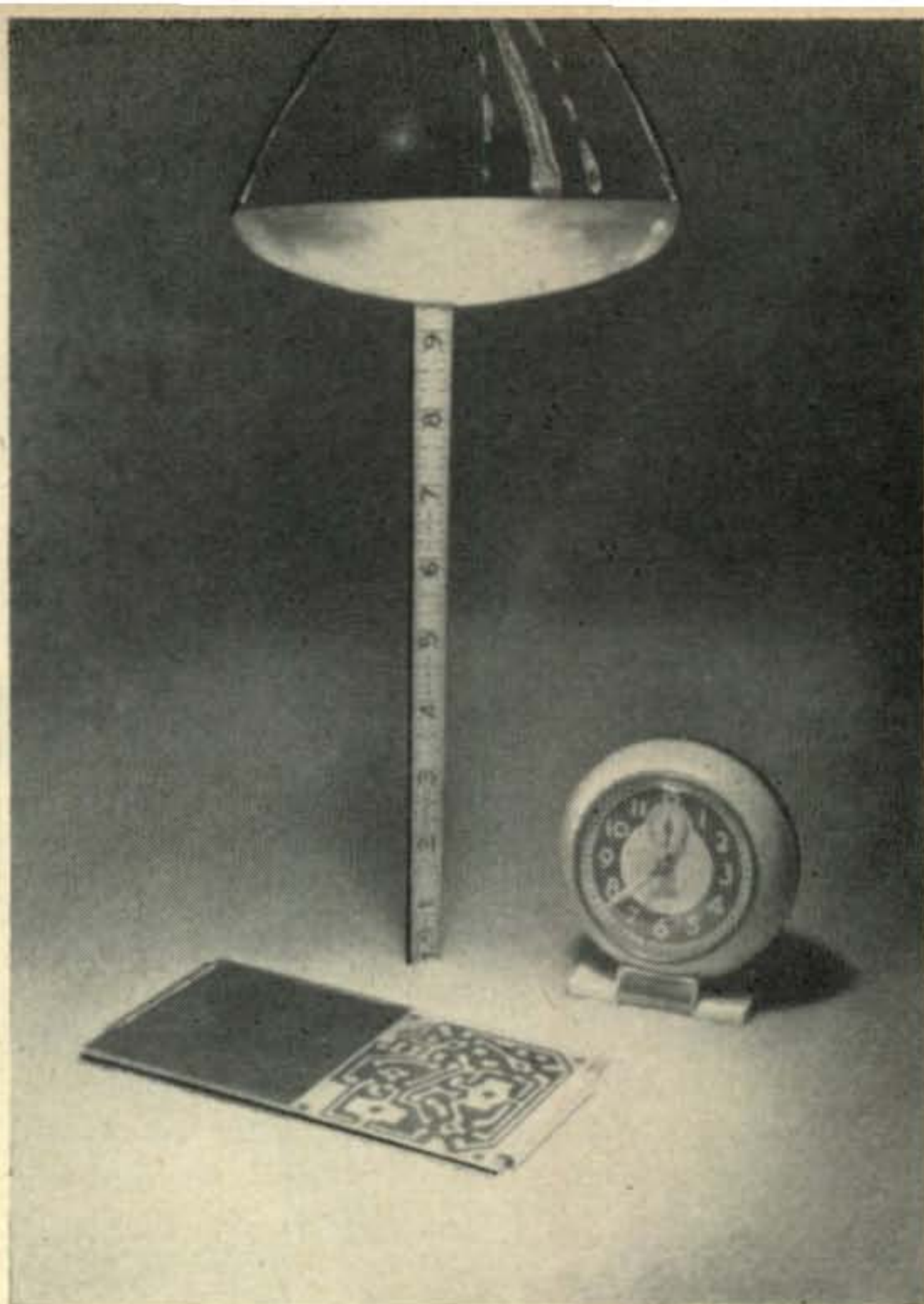
Fig. 8. Exposing to Harden Sensitized Surface
