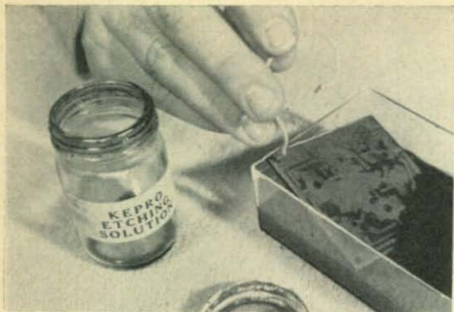
Fig. 11. Etching in Plastic Tray to Remove Unwanted Copper
