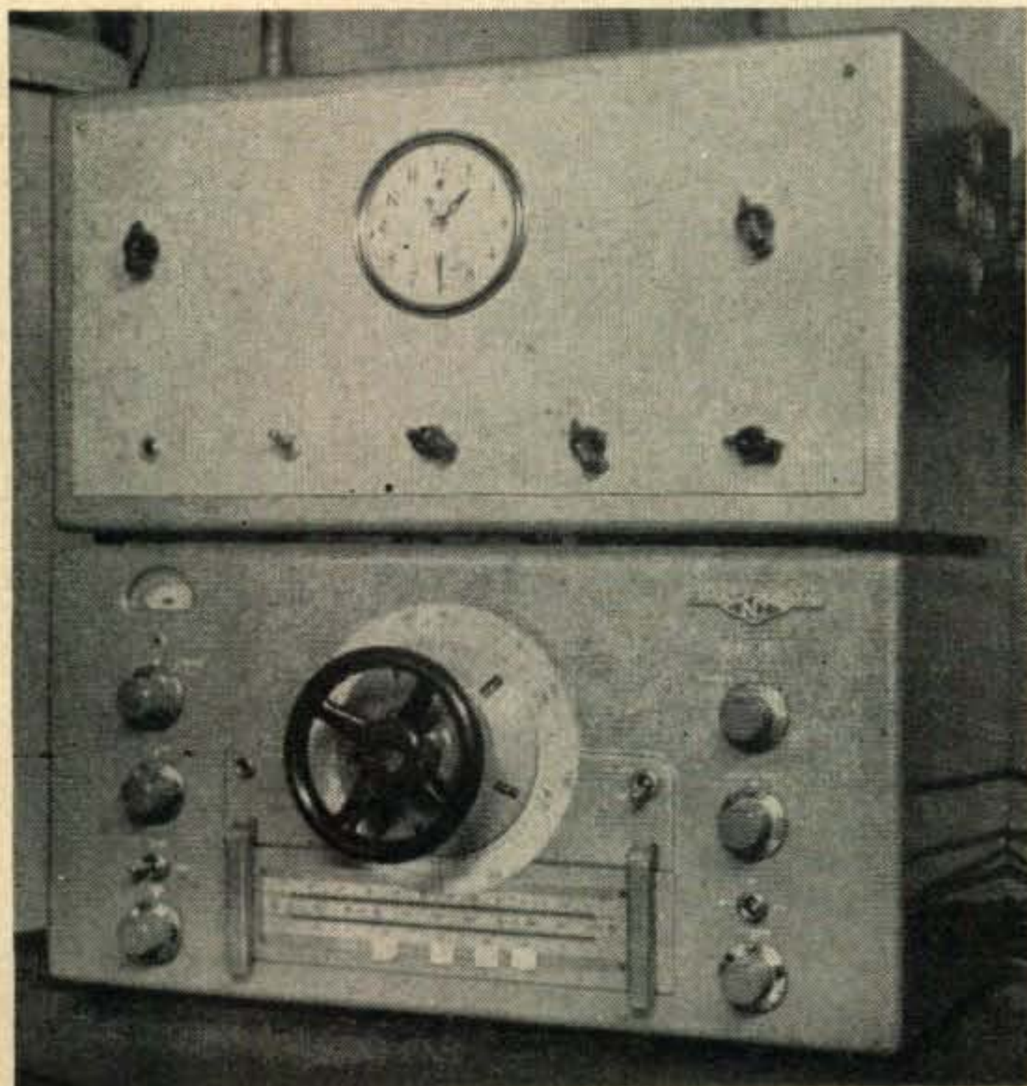
The author's receiver showing the oversize tuning dial.
